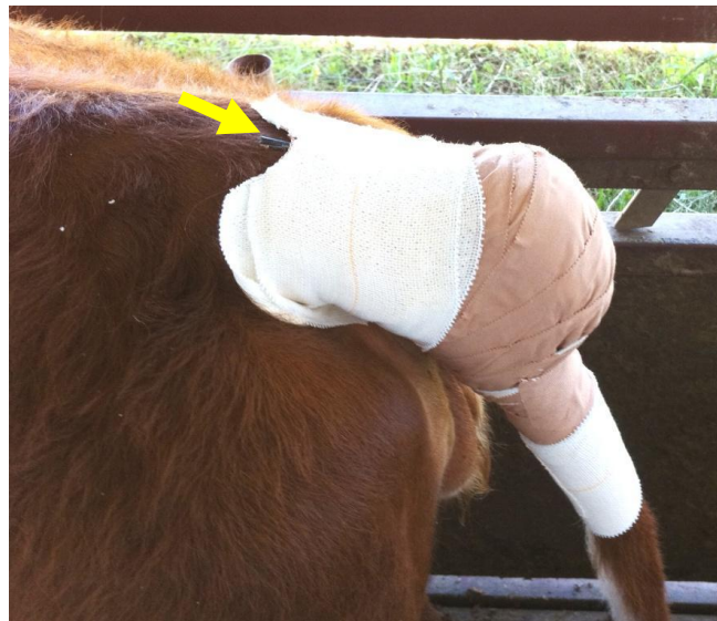
Figure 8. Data logger securely attached to the base of the tail of a heifer. Sensor probe arrowed
