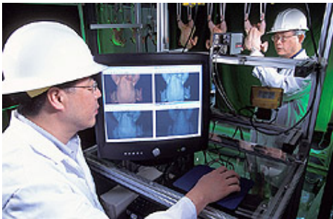
Agricultural engineers Kuanglin Chao (left) and Yud-Ren Chen discuss poultry carcass images taken with a multispectral imaging system. (K9936-1)
