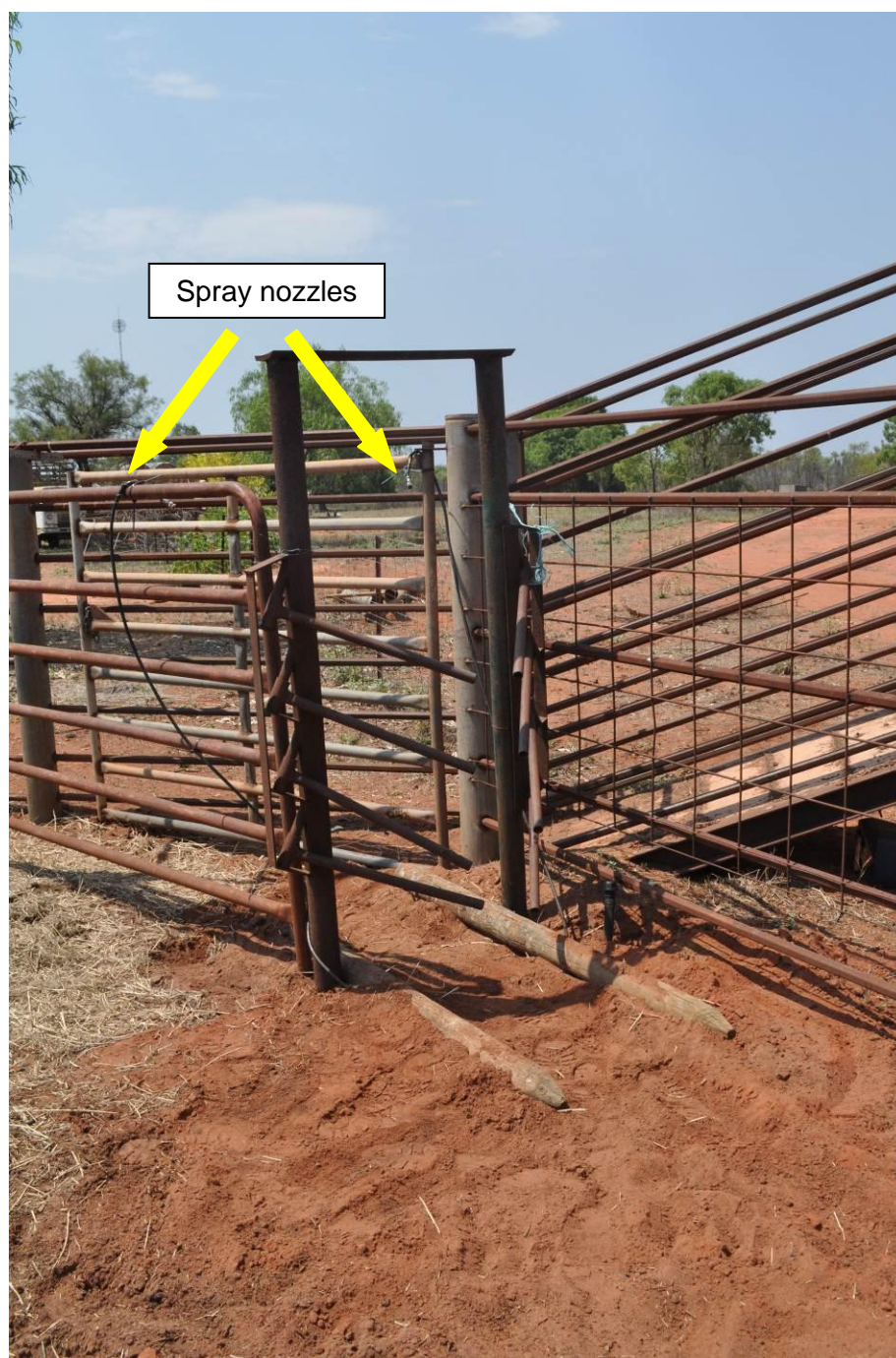
Photo 2 – The Tick Off system in situ. The trigger mechanism is buried between the two logs. The spray nozzles attached to the rails.
