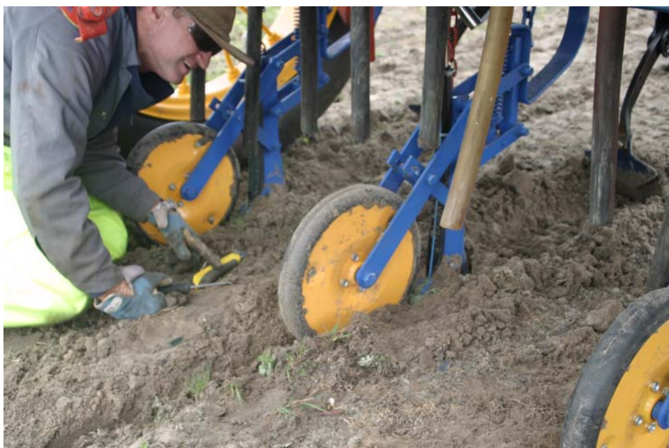
Figure 44. Tyne configuration on the DAFWA Massey Ferguson seeder.
