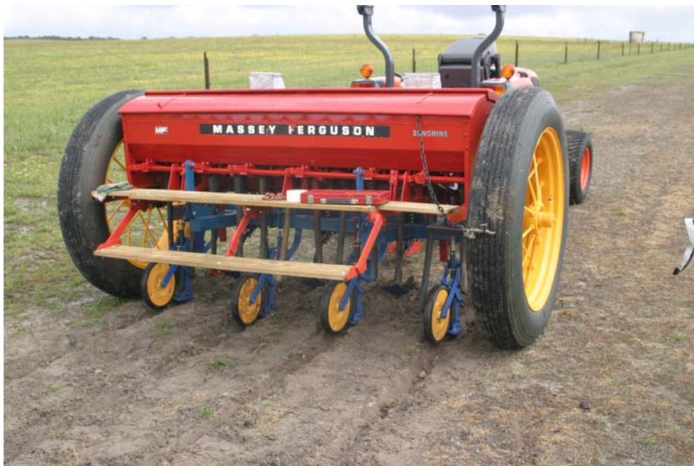
Figure 43. The renovated Massey Ferguson seeder adjusted to sow larger-scale paddock areas to perennial pastures.
