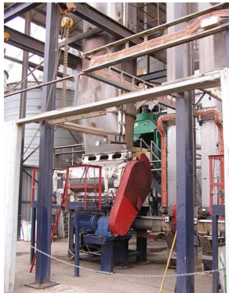
Photograph 4 – Typical steam flaker
