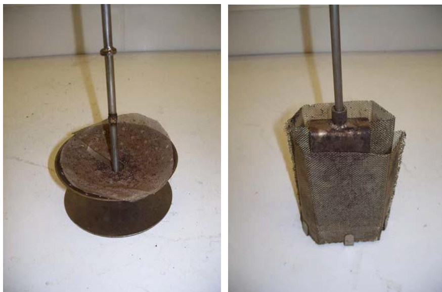
Figure 5. The two different baskets used in the basket rig. To the left the initial bowl-shaped basket and to the right the larger upright basket.
