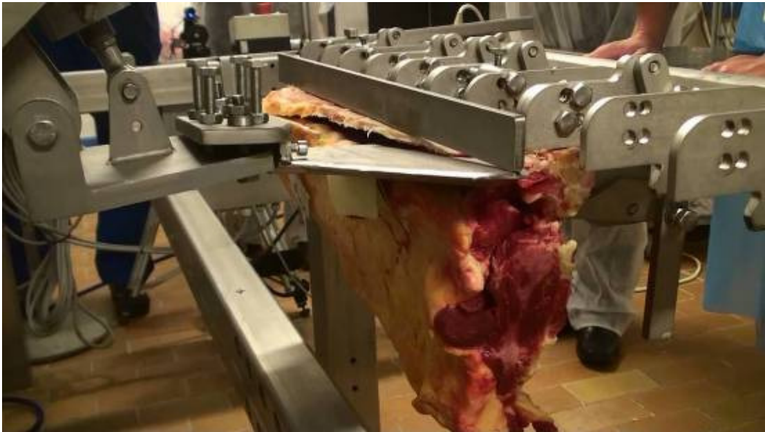
Figure 24 – Detail of successful cut with support plate
