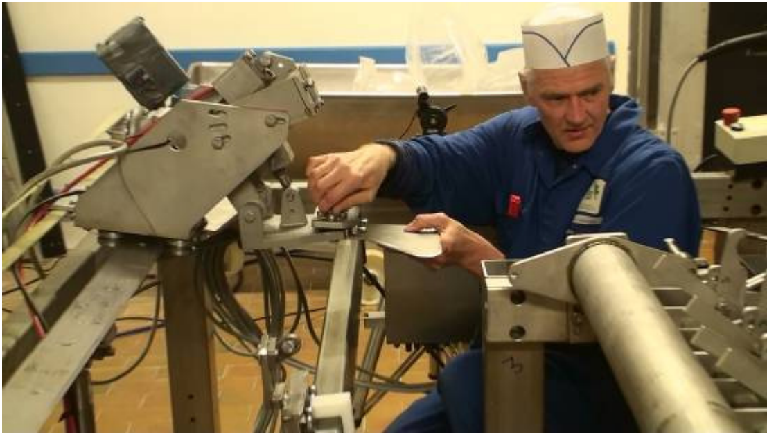
Figure 9 – Attaching the cutting plate to the work bench
