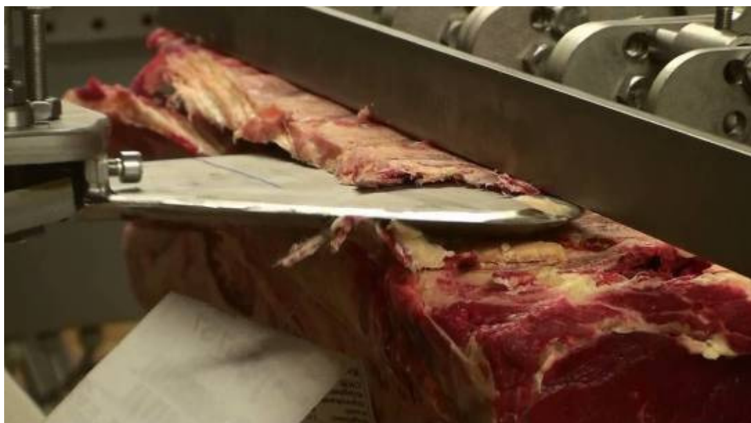
Figure 25 – Blade cutting through feather bone at cranial end
