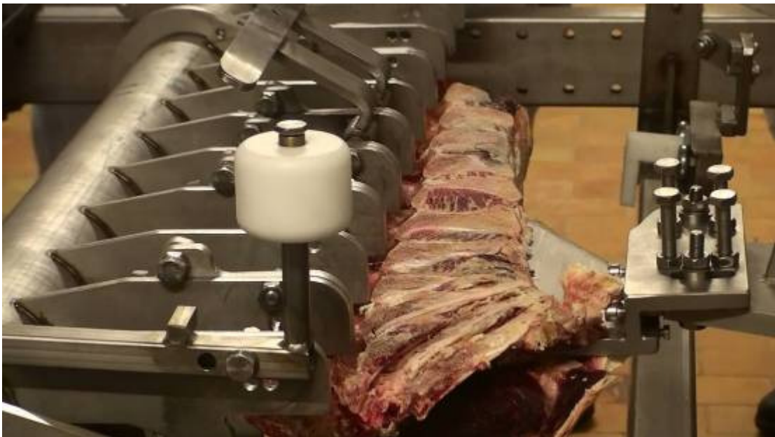
Figure 19 – Cutting plate deforming and detaching the feather bone
