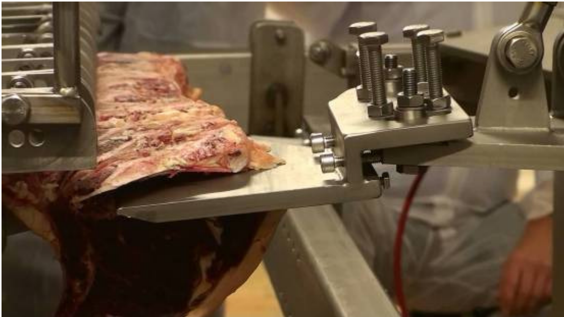
Figure 18- Cutting plate stuck against striploin
