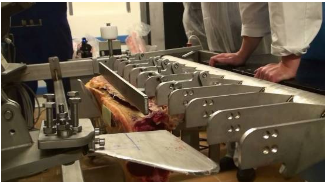
Figure 23 – First successful cut with support plate
