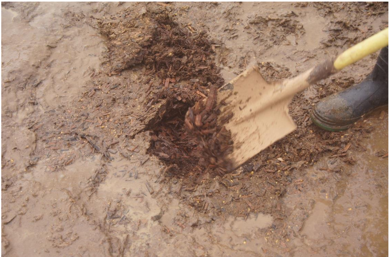
Photograph 10 – Woodchip bedding condition beneath the surface (Jan 2012)
