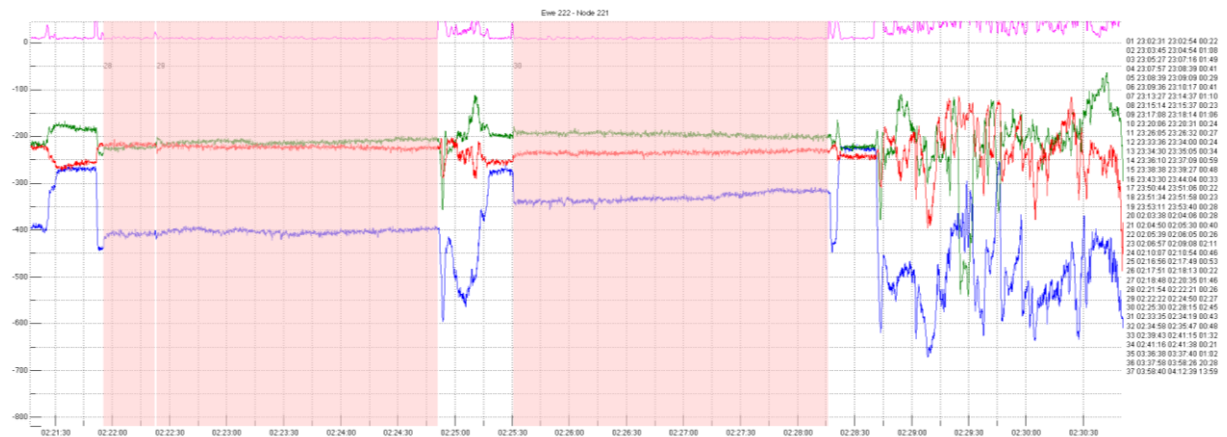
Figure 12: Three automatically classified stillness events. Green, blue and red traces are magnetometer data; pink bars indicate detected stillness events.
