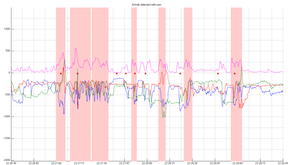
Figure 8: Automatically classified rotation events with the agitation index (Magenta trace). The red, blue and green traces are individual 3-axis magnetometer data; pink bands are detected circling/rotation events; red triangles are circling/rotation events identified by video annotation.
