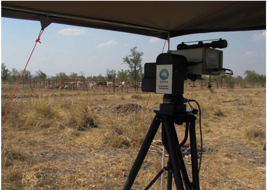
Fig. 1b Line averaged methane flux was determined using OPL at all sites.
