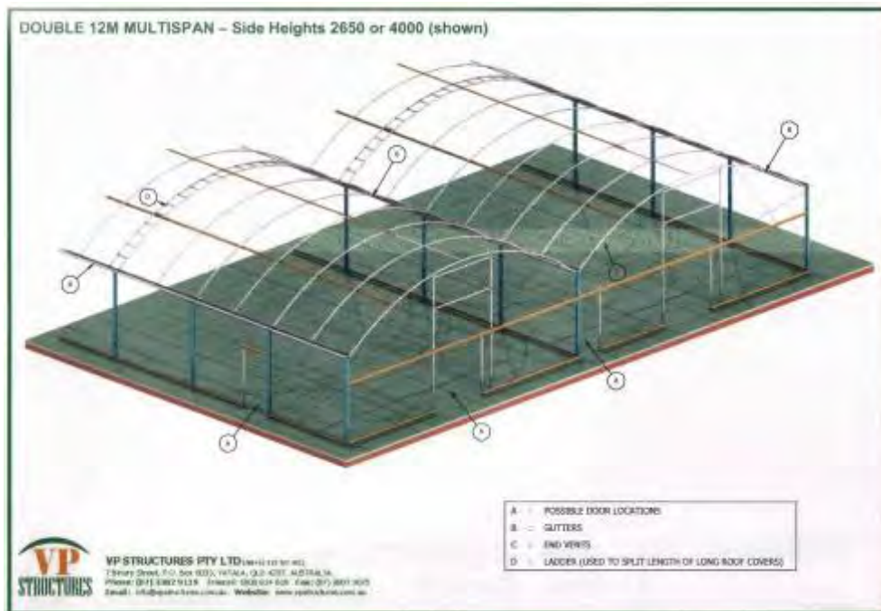
Figure 36 Semi-permanent lamb feeding shelter or double “eco-shelter design (Source: VP structures)
