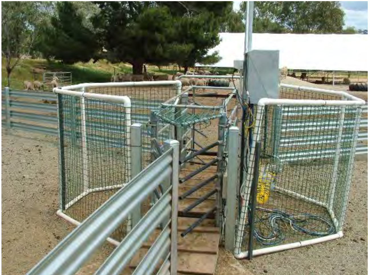
Figure 51 Walk through automatic weighing and drafting system (Courtesy: R. Shepherd Sheep CRC)
