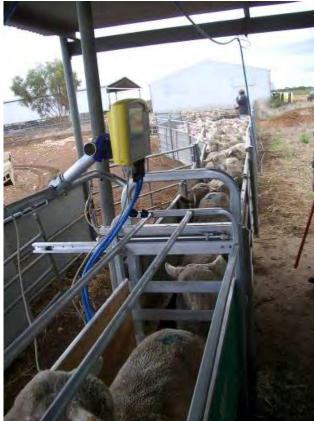
Figure 49 Automatic drafting and weighing system for sheep and lambs (Source: Productive Nutrition Pty Ltd)
