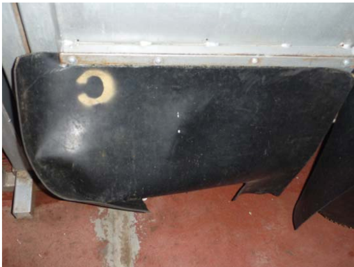
Figure 02: Rubber skirting material on the Mark 4 restraining box
