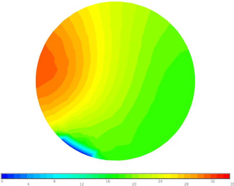
Figure 5: Voltage gradient in cross section using 10 Ω.m skin resistivity.
