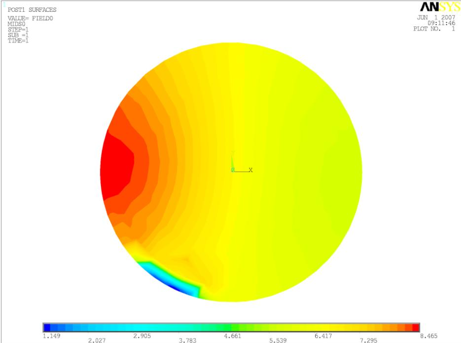
Figure 6: Voltage gradient in cross section using 75 Ω.m skin resistivity. The results of the simulations are shown in the tables below. The two critical columns are Vh – voltage exposure during contact with the carcass – and Ec – the gradient through the core and, hence, effectiveness at immobilisation.
