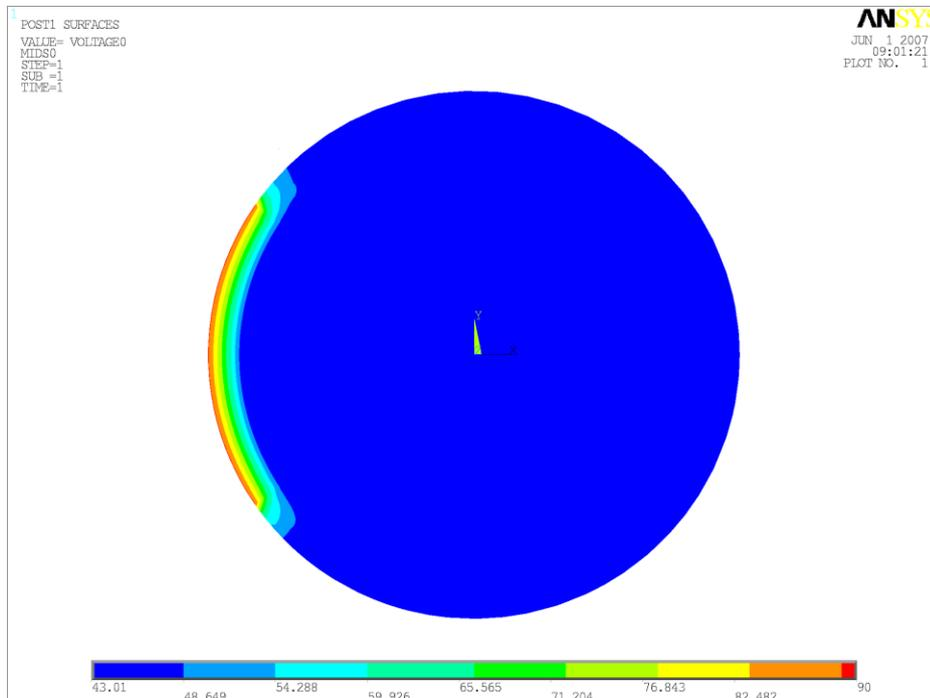
**Figure 3** - Contour plot of the voltage through a cross section of the carcass at the site of the live electrode.
