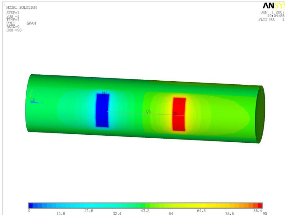
**Figure 4:** Carcass surface voltages.
