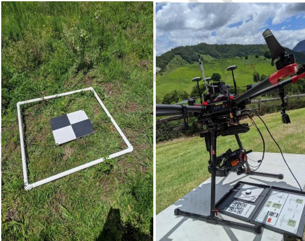
Fig. 5. (left) Placement of a Ground Control Point (GCP) at Nobbys Creek. A minimum of five GCPs must be placed across the extent of the surveyed area. (right) Collection of white reference at Nobbys Creek to correct atmospheric disturbances in spectral imagery.
