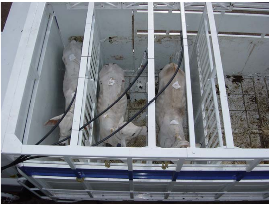
Figure 29. Sentinel steers in individual pens. Note the black piping that carried the catheter lines into the cabin of the truck to facilitate blood sampling while mobile.
