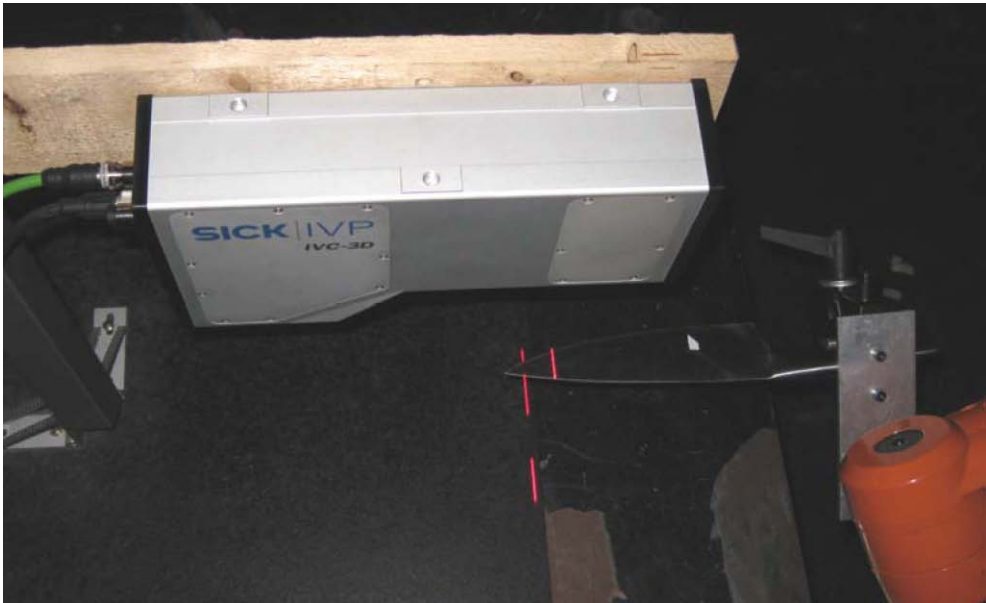
Figure 9. Sick IVP IVC 3D sensor inspecting a blade moved by a robot.
