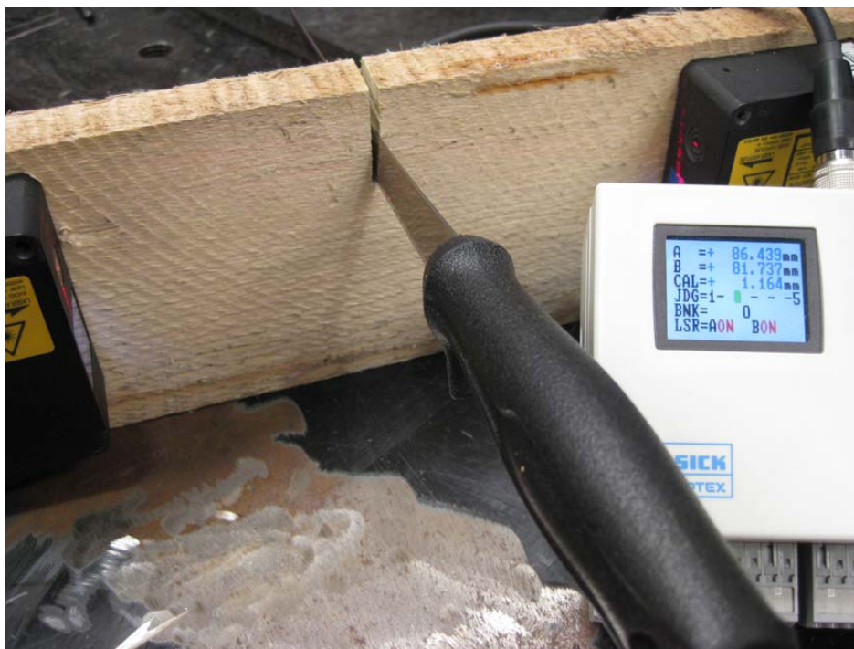
Figure 8. Laser Distance Thickness Profiling
