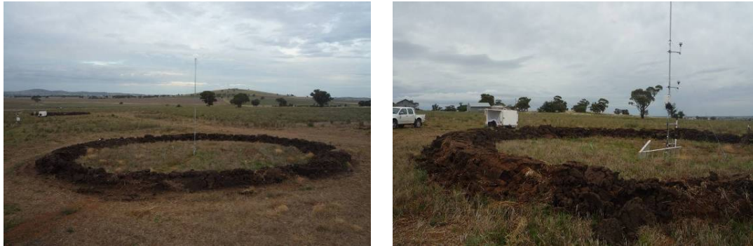
Figure 1 L: UI-treated (foreground) manure rings at the summer 2011 field site. R: Sampling mast of untreated ring (at centre) also includes vertical array of five 2D sonic anemometers.
