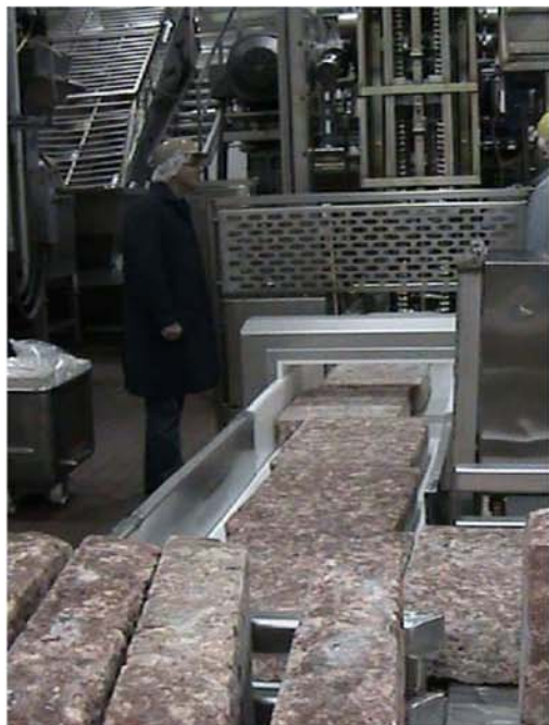
Blocks fed via metal detector to vertical elevator for No. 2 grinder
