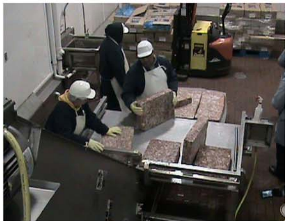
Blocks being fed onto inclined conveyor
