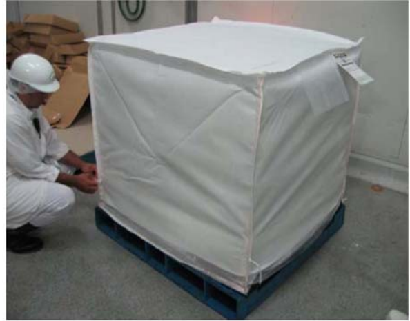
Polypropylene top being secured to base
