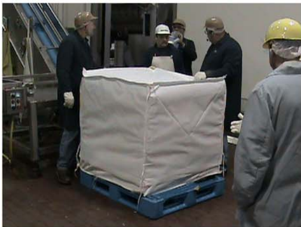
Unit to be opened for grinding. Inclined conveyor to No. 1 grinder in background
