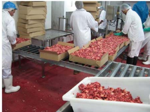
Cartons being levelled, filled to weight and lidded
