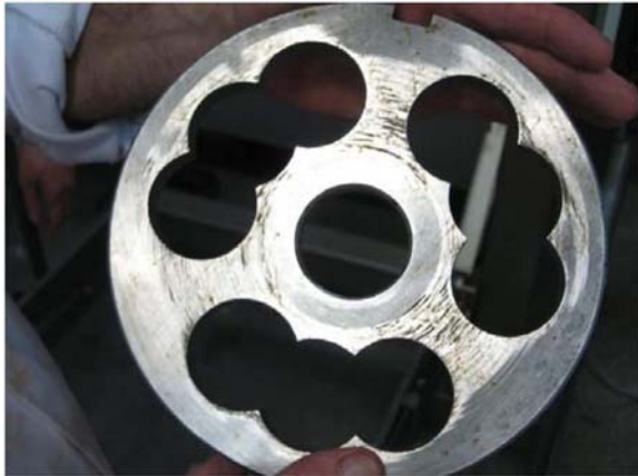
Kidney plate used in grinder – 40 mm holes
