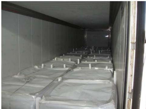
Shipping units (20) loaded into container with dunnage strips of polystyrene
