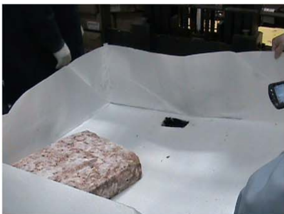
Evidence of fork puncture of polypropylene base
