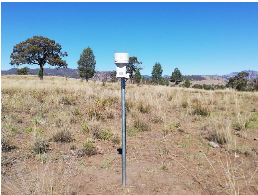
Figure 3-8: Rain Gauge Installation
