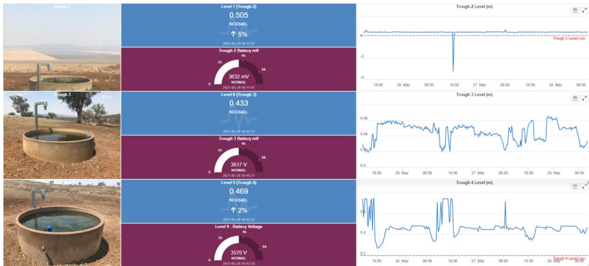
Figure 4-1: Trough water level dashboard
