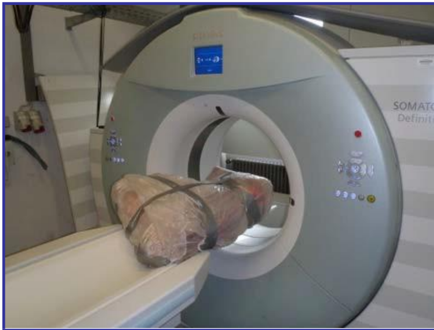
Figure 8: Beef packaged for fan beam scanning.
