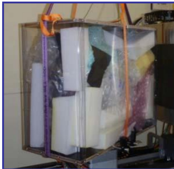
Figure 7: Beef packaged for cone beam scanning.
