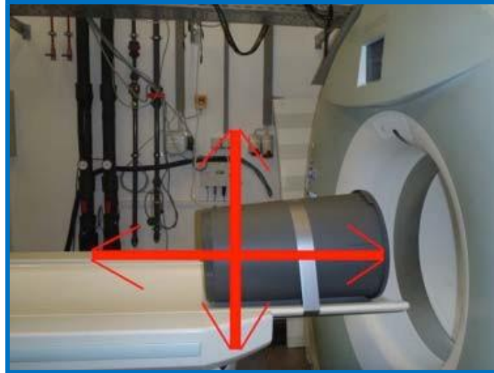
Figure 13: Directions of platform movement.
