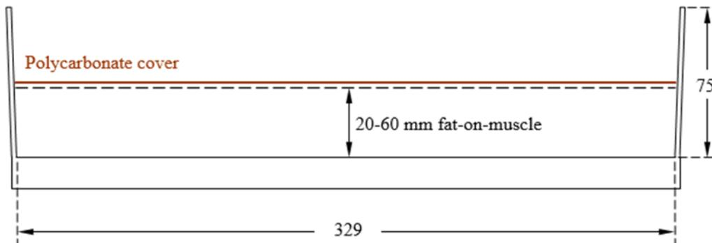
Fig. 13: PVC former and muscle/fat fill for phantoms.
