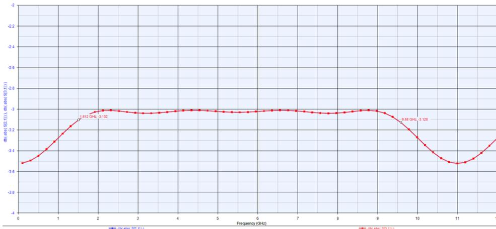
Fig. 5: Insertion loss for the schematic level simulation of the power divider.
