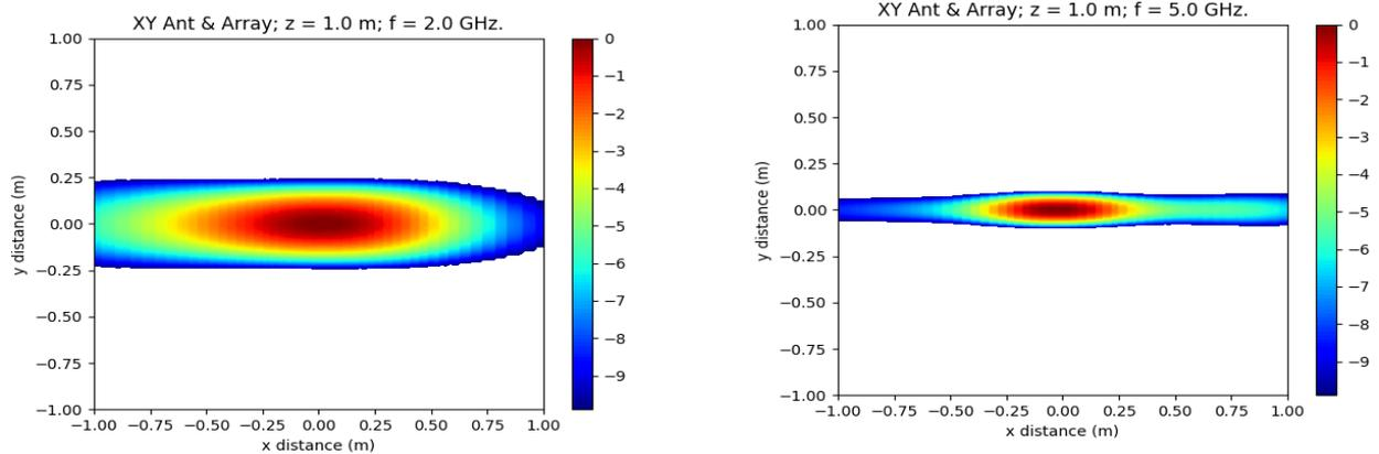
Fig. 12: Antenna array footprint size at 1m and for 2 and 5 GHz.
