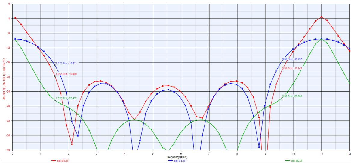
Fig. 4: Return loss and isolation for the schematic level simulation of the power divider.
