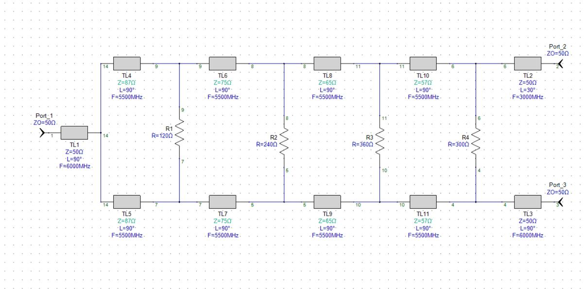
Fig. 3: Schematic level simulation of the power divider.
