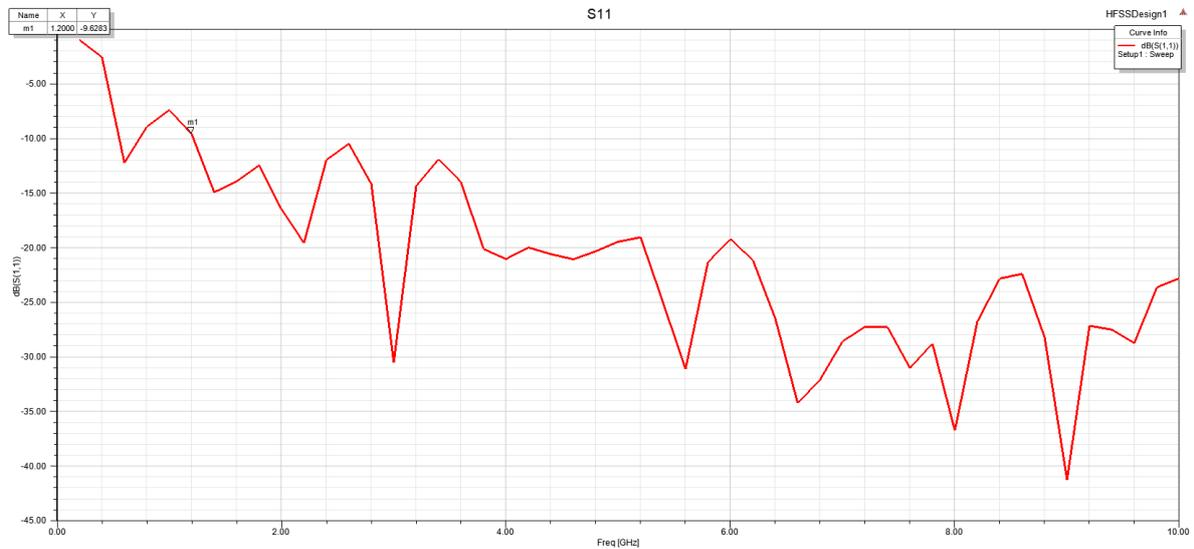
Fig. 1: Simulated S11 of the antenna indicating that antenna operation starts at 1.2 GHz.
