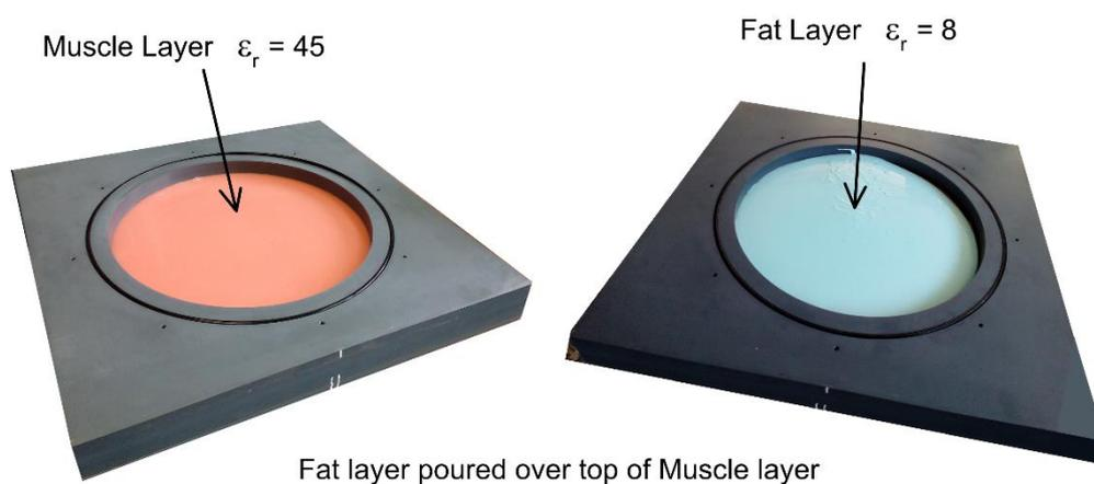
Fig. 14: Phantom target #3 – 1.9 cm fat layer poured over the top of a muscle layer.
