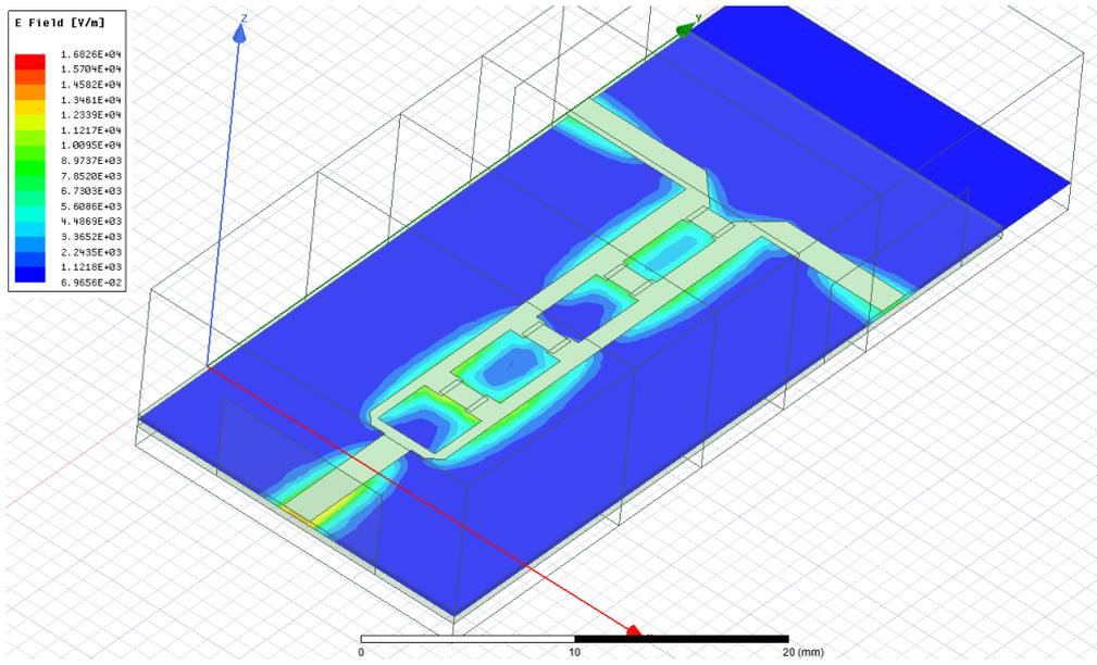
Fig. 6: Typical electrical field strength for the power divider.
