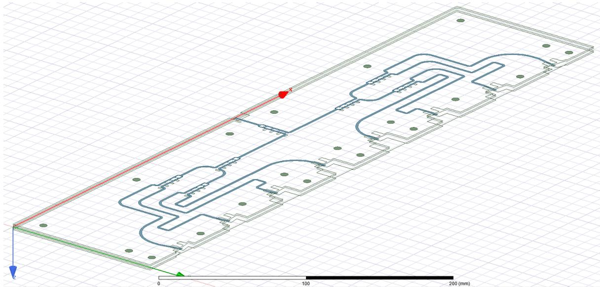
Fig. 11: Feed structure design fabricated on a PCB.
