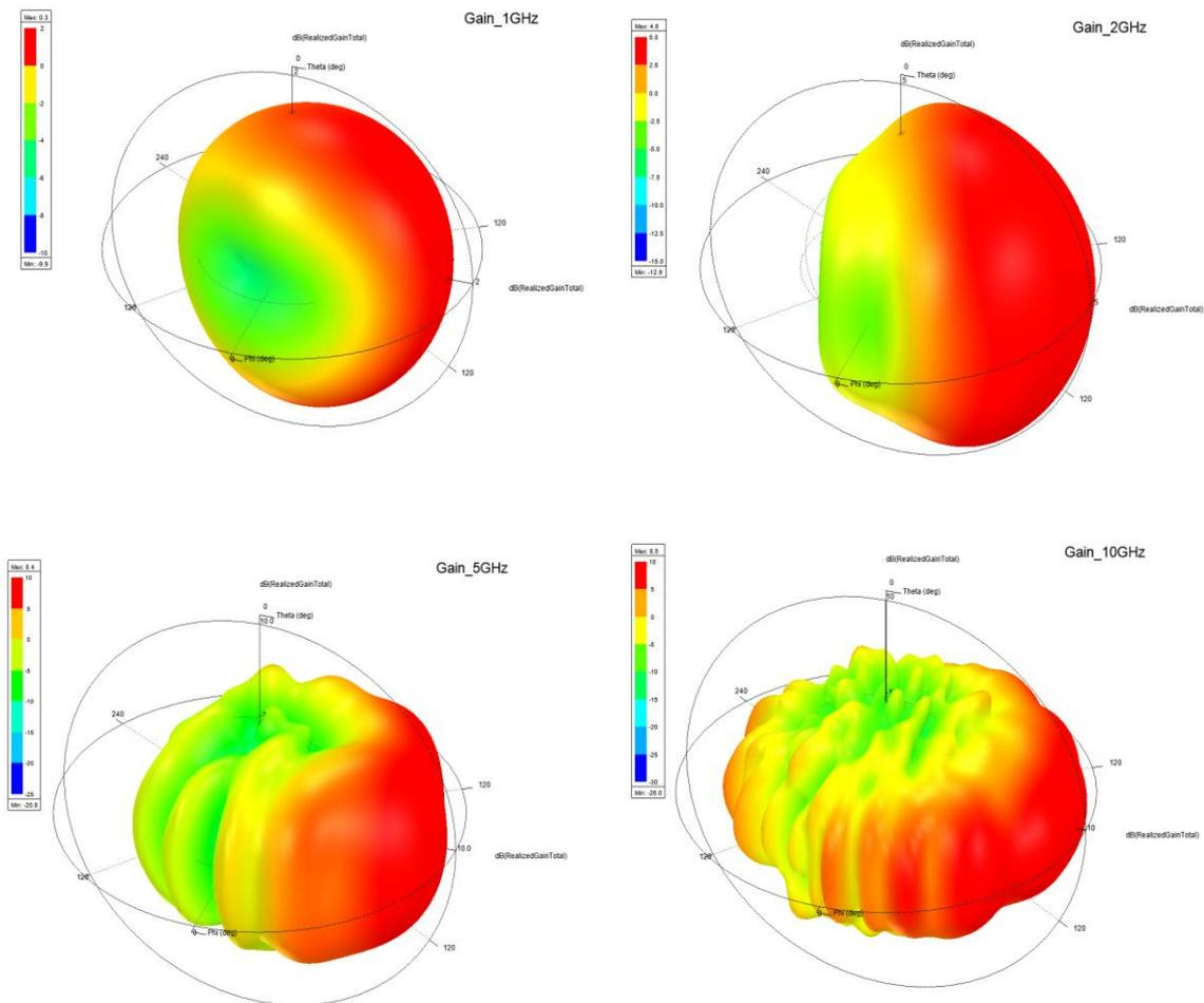
Fig. 2: Simulated radiation patterns show that antenna achieves a good main lobe in radiation patterns for all frequencies within the operating range.
