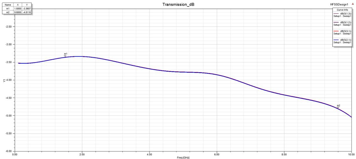
Fig. 9: Simulated results for insertion loss for the case of copper conductor and dispersive dielectric in the power divider.
