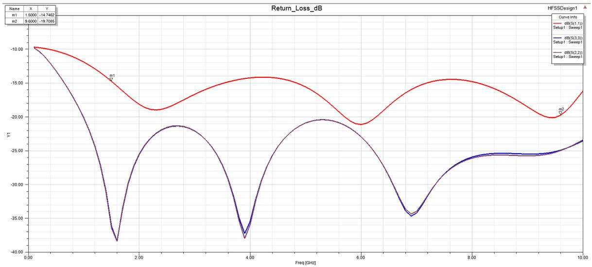
Fig. 7: Simulated results for return losses in the power divider.
