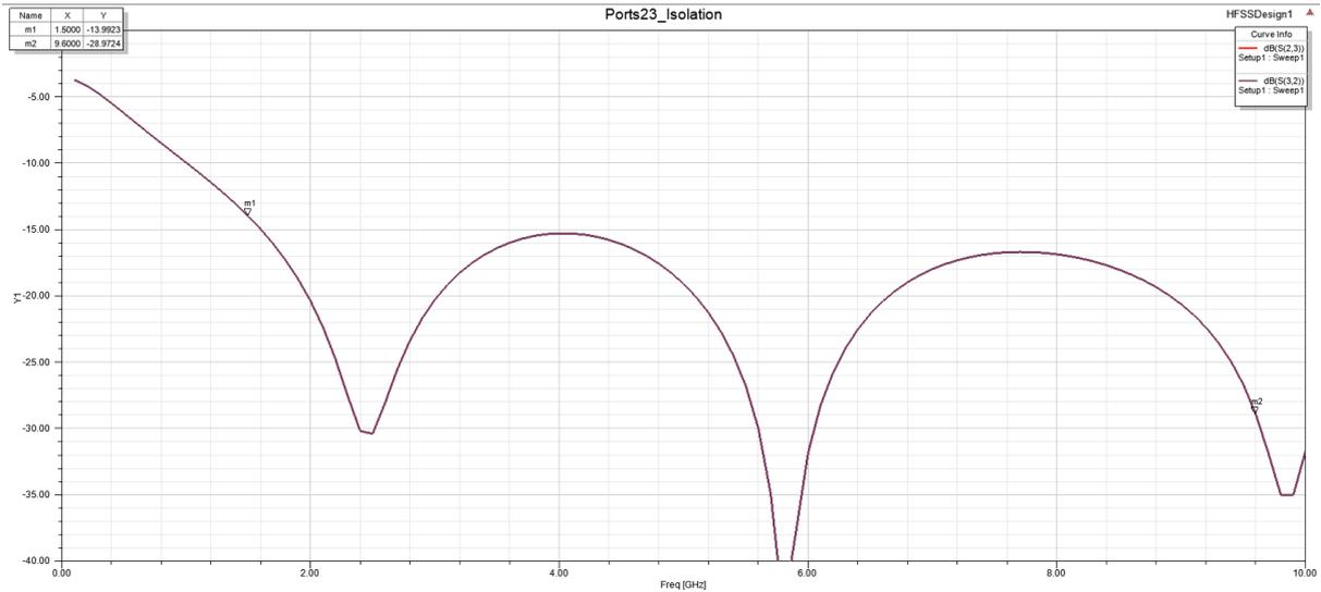
Fig. 8: Simulated results for isolation in the power divider.
