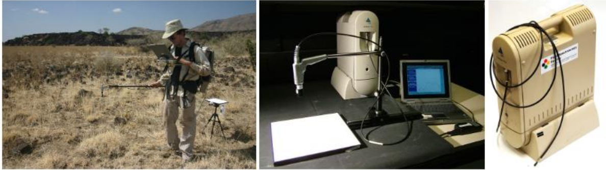
Figure 1.1 ASD FieldSpec Pro System (pictures obtained from the ASD website).
