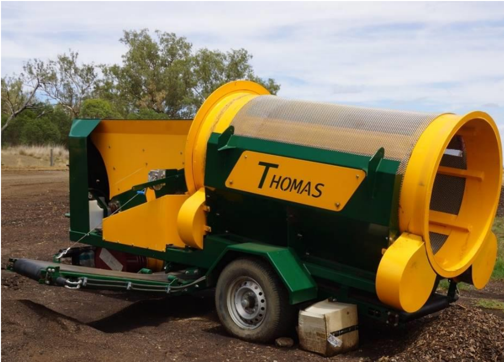
PHOTOGRAPH 54 – A TROMMEL (ROTATING SCREEN)
