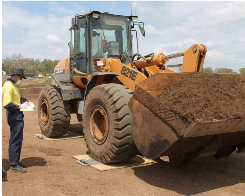
PHOTOGRAPH 66 – RECORDING LOADS BY WEIGH PADS DURING SEPARATION TRIAL
