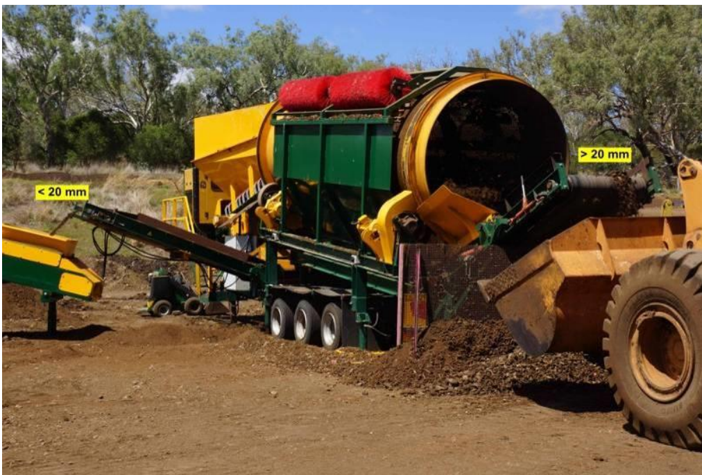
PHOTOGRAPH 68 – TROMMEL WITH A 20 MM SCREEN USED AT TRIAL SITE
