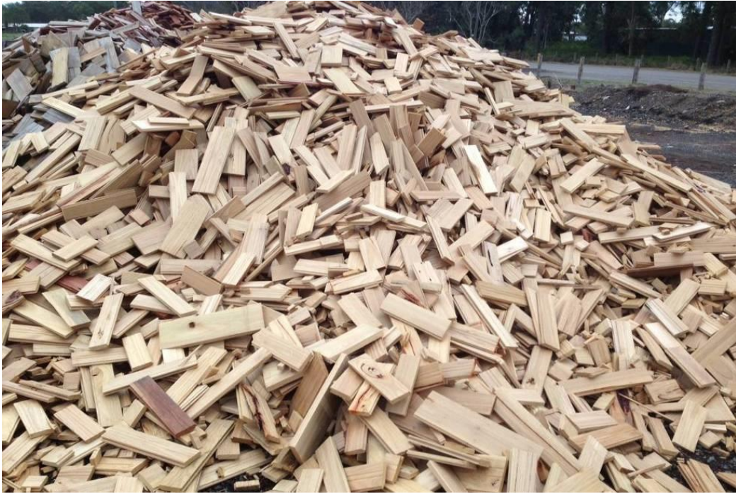
PHOTOGRAPH 11 – BEDDING OPTION – TIMBER OFF-CUTS
