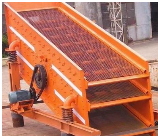
PHOTOGRAPH 55 – AN EXAMPLE OF VIBRATING SCREENS
