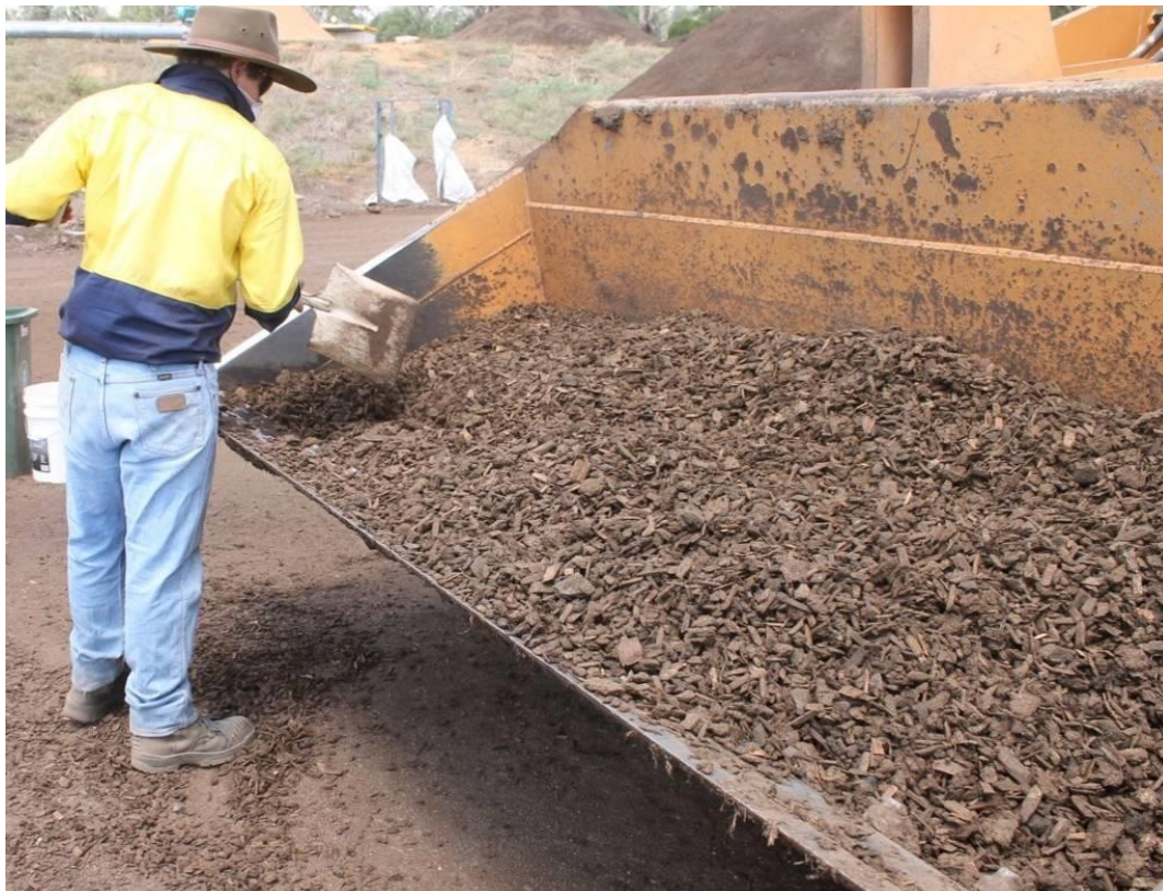
PHOTOGRAPH 73 – MANURE AND WOOD CHIPS SCREENED FROM VIBRATING SCREEN - 10 TO 40 MM
