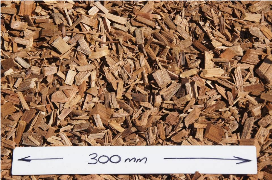
PHOTOGRAPH 15– TYPICAL WOOD CHIP
