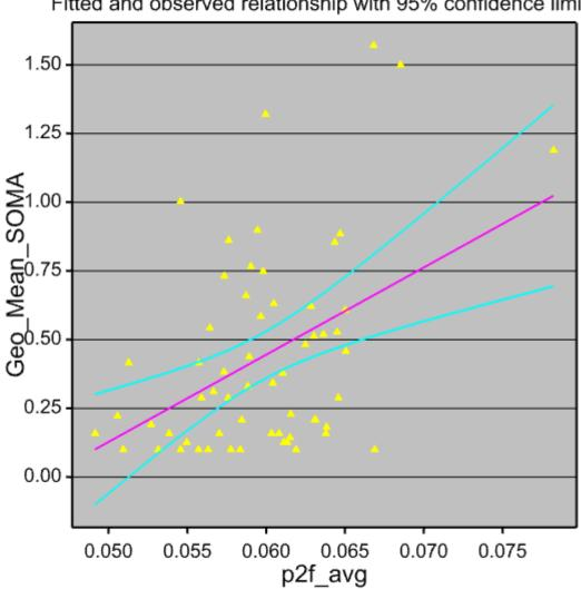
Figure 5. The geometric mean SOMA IMF versus NMR determined IMF on 60 thawed loin muscles (Geometric mean SOMA =  $-1.46 (\pm 0.515) + 31.7 (\pm 8.59) * NMR p2f, R^2 = 0.177$ , p<0.001).
