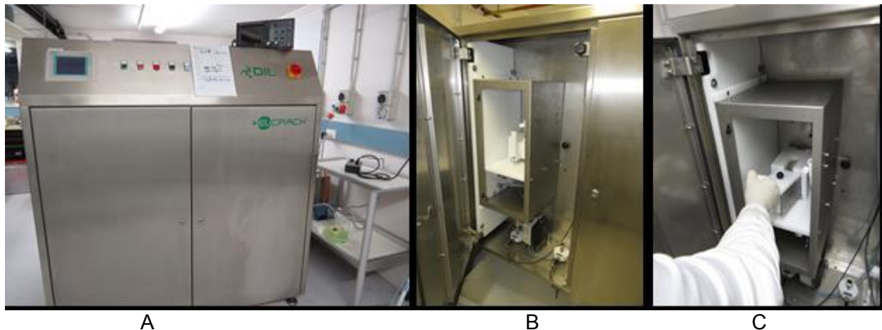
Figure 1. Pulsed electric field system (Elcrack- HPV5, DIL, Quakenburck, Germany) used in the present research. A) the front of the instrument showing the control panel, B) the back of the instrument and C) the treatment chamber housed between the electrodes.
