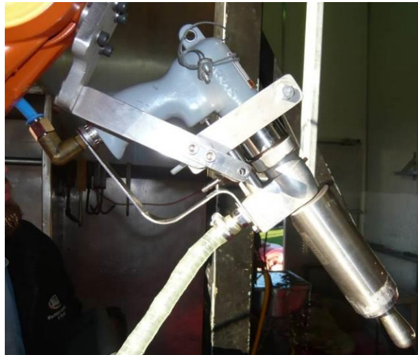
Fig.5 Jarvis Manual Bung Cutter mounted to robot
