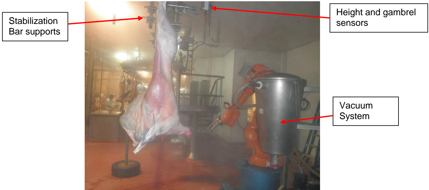
Fig.26 Online Robot Trial setup at GMP June 2012
