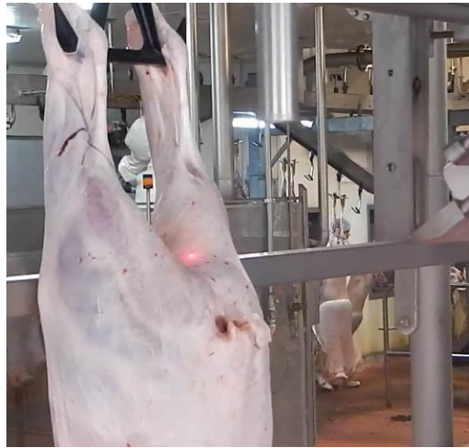
Fig. 50 Carcass that resulted in a good cut, red laser dot for height detection can be seen
