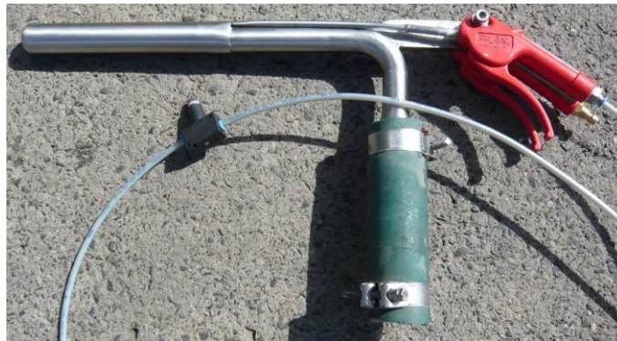
Fig.10 Top view of modified Manual Evacuation tool showing 'Pistol Grip' valves welded into outer tube.
