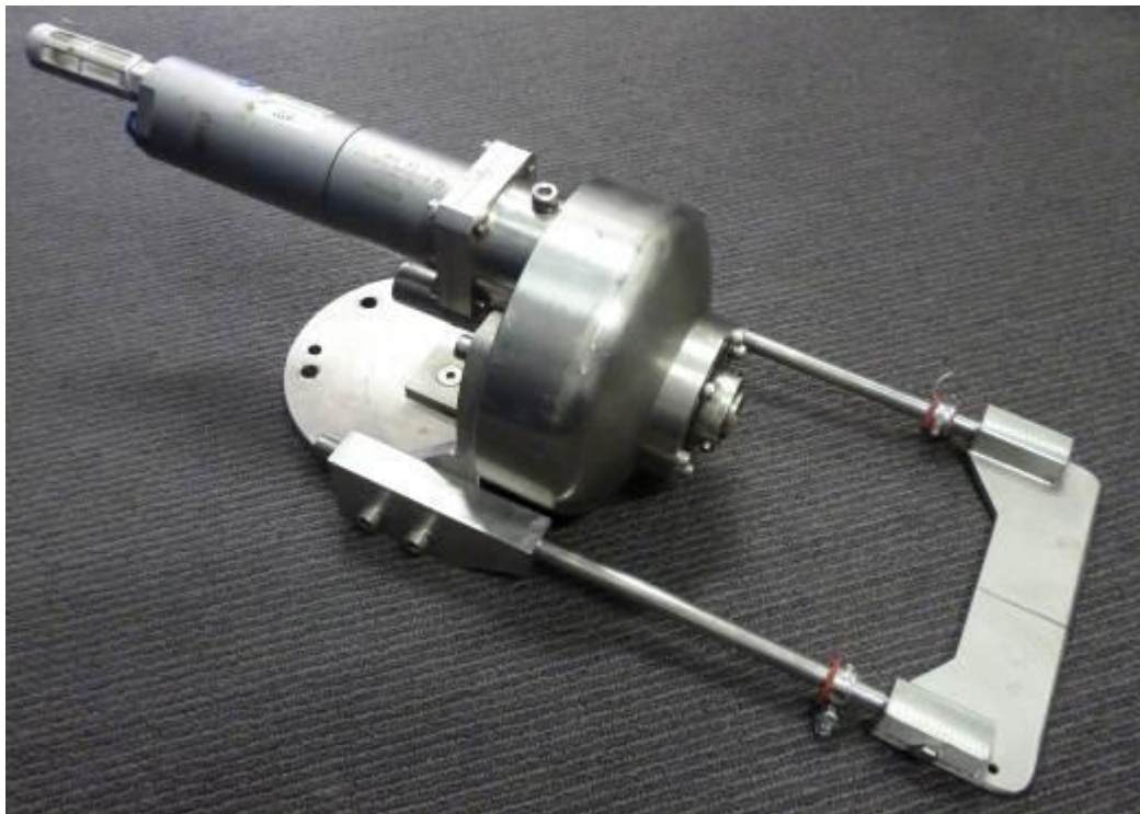
Fig.29 Upgraded Tail manipulator, tool shown with cutter removed.
