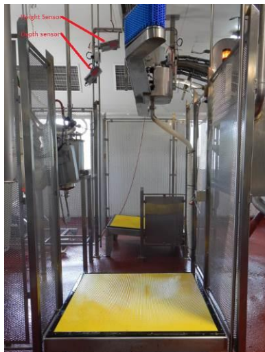
Fig. 53 The two Optical Sensors used, one detecting crotch height one detecting the thickness of the carcass in the bung region.
