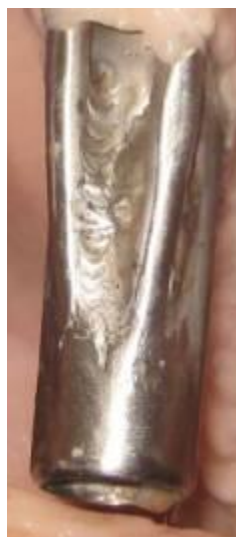
Fig.6 Manual Evacuation tool with air and water tubes welded to outside of the tube.
