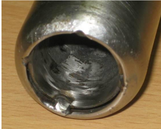
Fig.9 Modified 'nose' of manual evacuation tool
