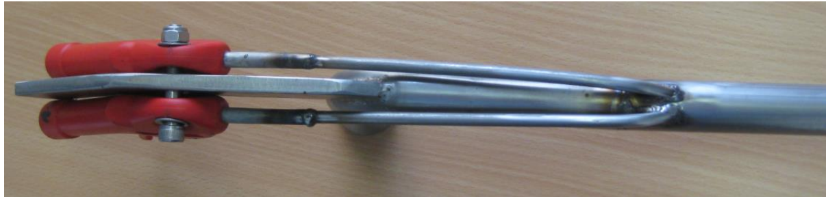
Fig.10 Top view of modified Manual Evacuation tool showing 'Pistol Grip' valves welded into outer tube.
