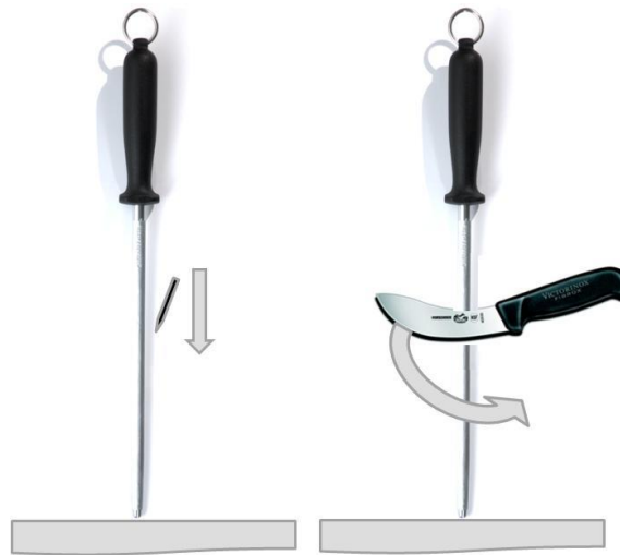
Figure 7.6: Holding the steel still and vertically to sharpen the knife
