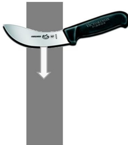
Figure 7.5: Sharpening the knife by using a slicing action with the edge
