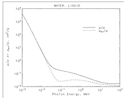
Figure 2 - Absorption coefficient graph for water
