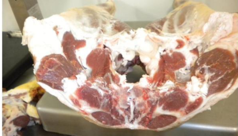
Figure 34: Lamb hindquarter cut with the ROC Automated primal cutting system, note cut meat surface and lack of bone dust present.
