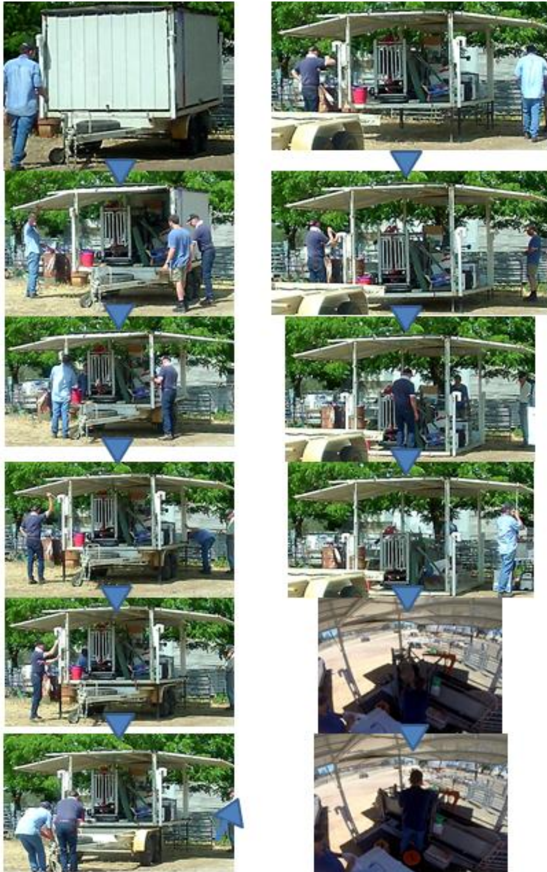
Figure 3 Flowchart of changing “Bush-Tiger Milker” from travel mode to working mode
