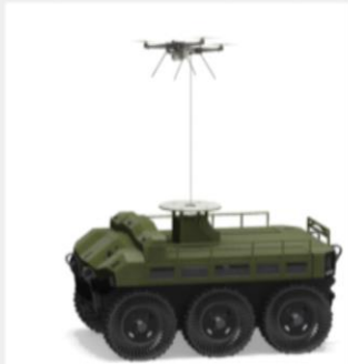
Drover WOLF can autonomously fly a tethered quadrotor to count livestock, assess pasture health, or detect pest animals.
