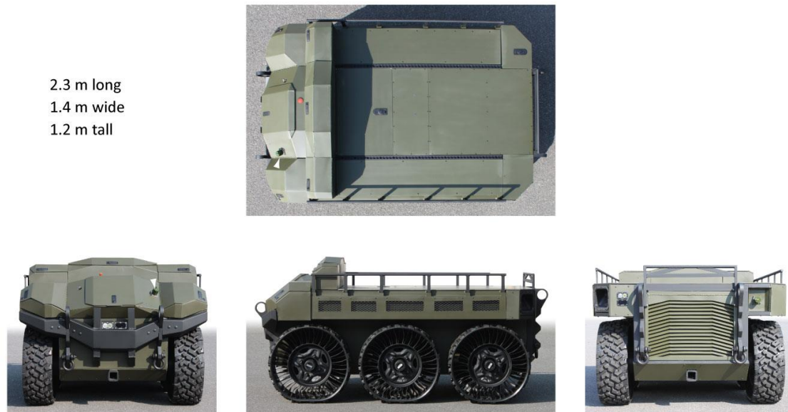
Figure 4: HDT's Drover WOLF unmanned vehicle is about the same size as a large quad bike, but far more powerful and stable.
