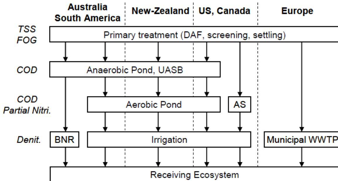
**Figure 2: Principal wastewater treatment set-up of the meat industry [3]. Note: At some smaller Australian plants, primary treatment may be bypassed and/or raw effluent may be used for irrigation or land application.**
