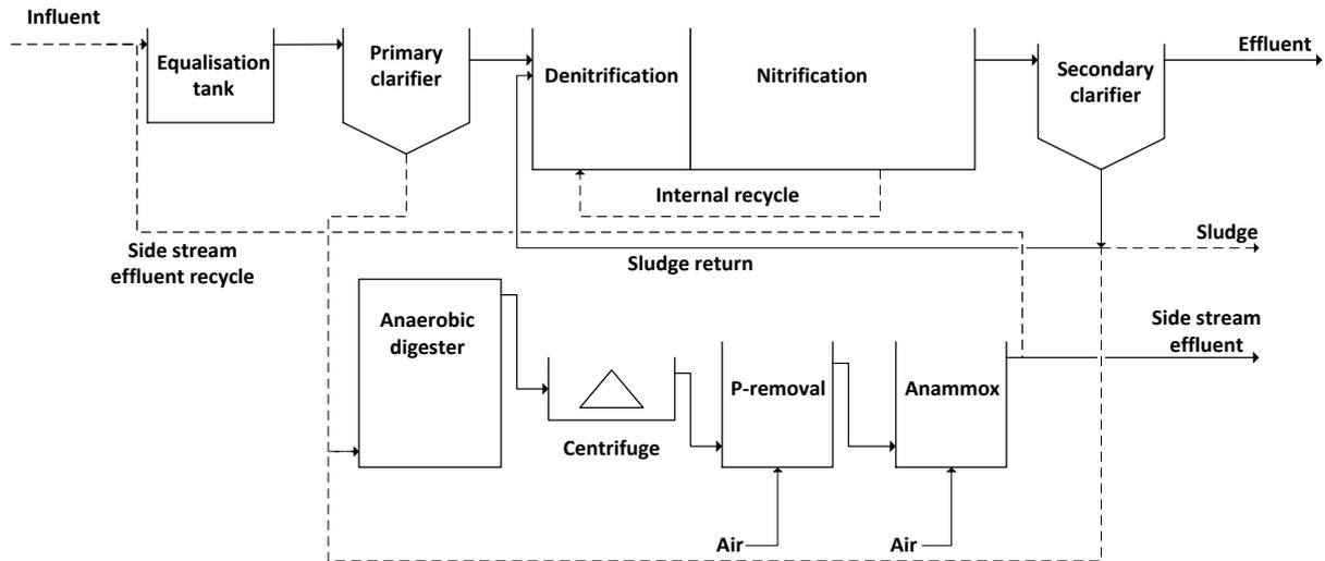
Figure 9: Schematic representation of conventional activated sludge treatment with side-stream treatment.
