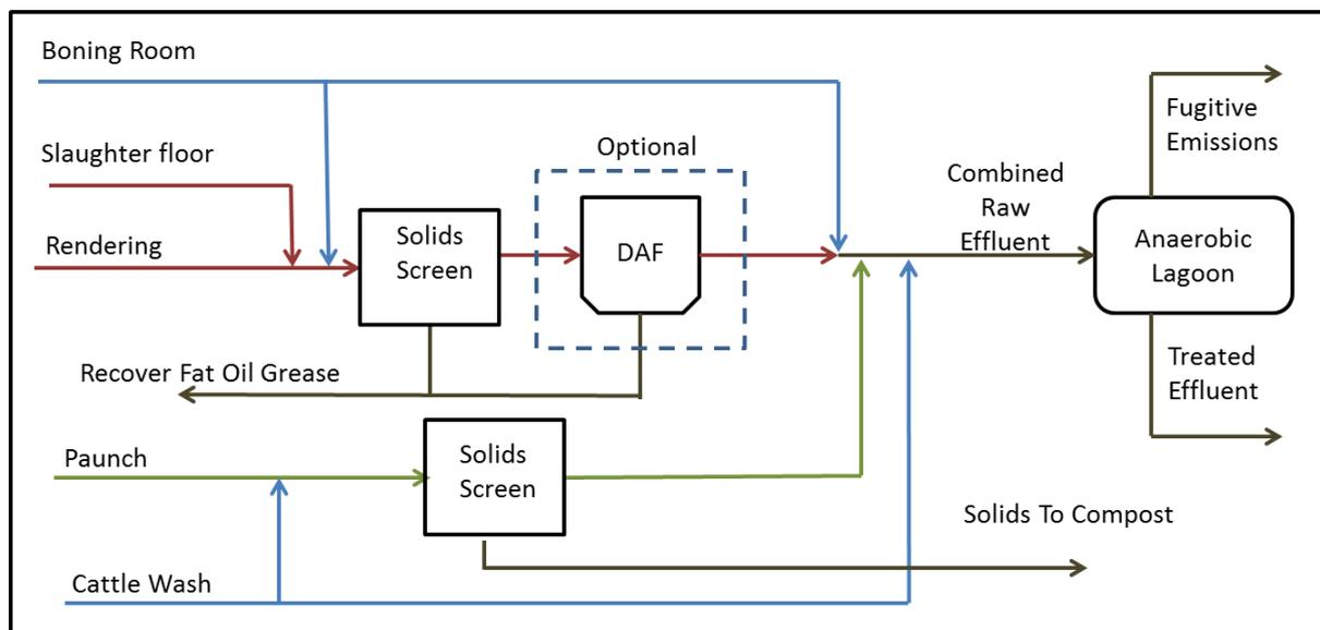
Figure 1: Major wastewater sources and generalised structure of waste and wastewater handling practices at Australian red meat processing sites
