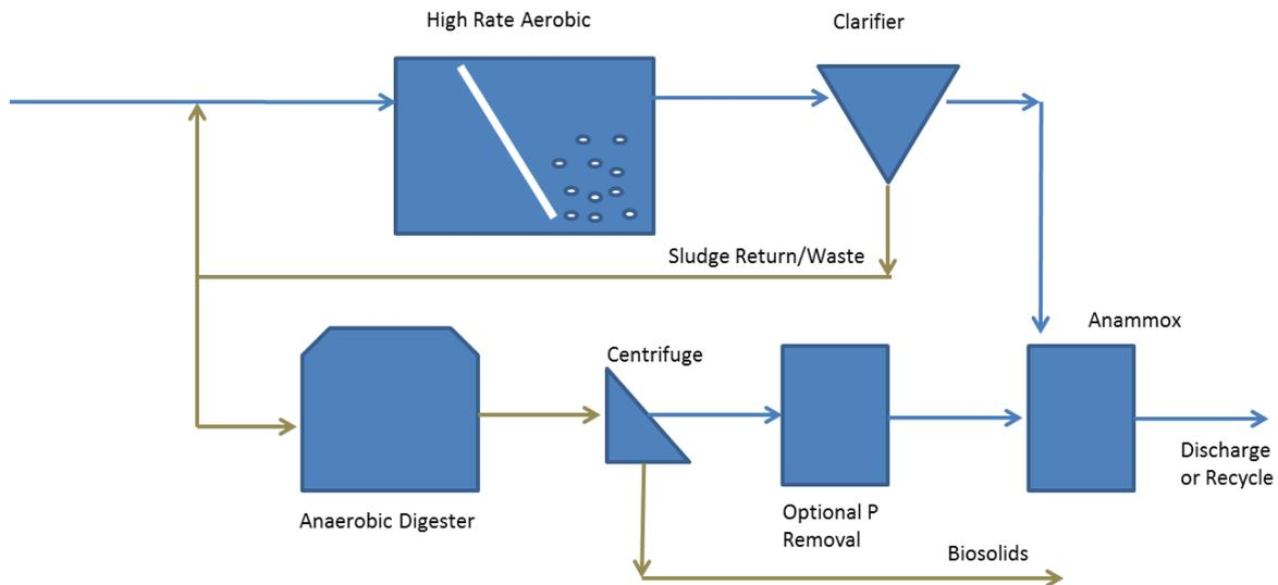
**Figure 22: High rate aerobic wastewater treatment and anaerobic digestion with anammox integrated for treatment of side stream AD centrate (A.ENV.0150)**
