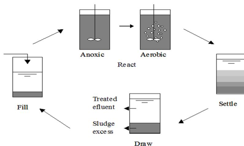
Figure 13: Principal operating modes of a Sequencing Batch Reactor (SBR) – Note: all stages occur within a single reactor.
