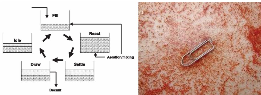
**Figure 8: Principal phases of a SBR (left)<sup>7</sup> and the biomass content of the DEMON® technology (right)**
