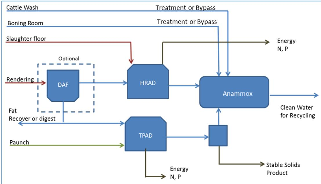
Figure 17: Separation of wastewater streams based on similar properties with primary treating using anaerobic digestion and potential anammox for treatment AD centrate (A.ENV.0151)
