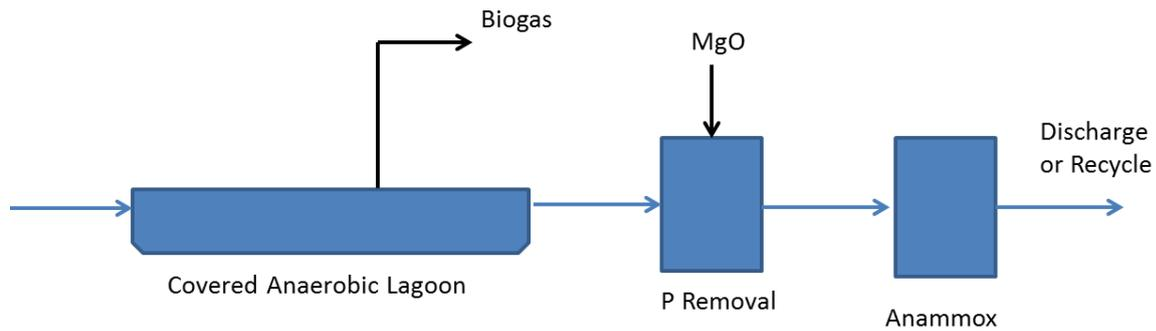
**Figure 20: Process flow sheet representing covered anaerobic lagoon followed by anaerobic ammonium removal; Phosphorus removal is optional and is not included in cost calculations.**
