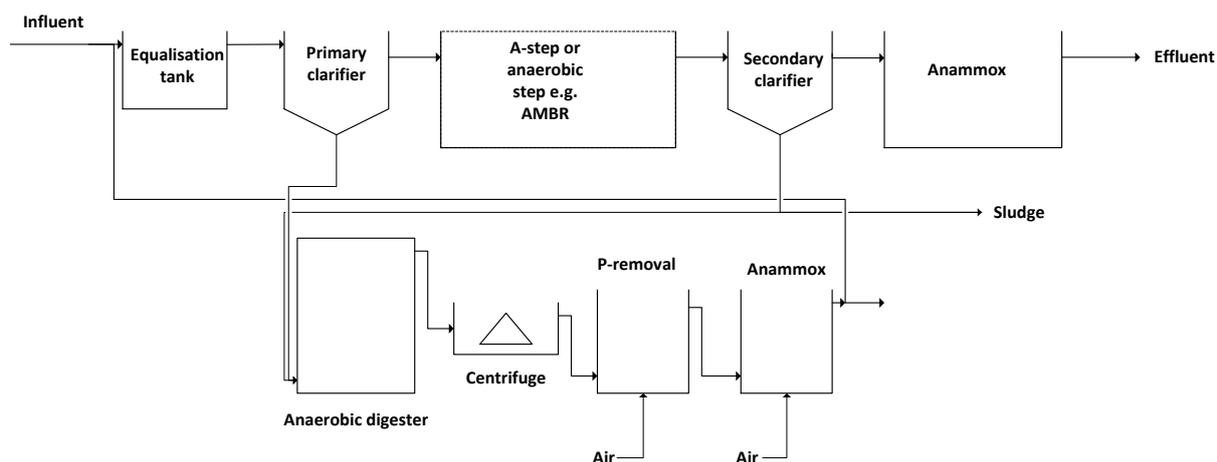
Figure 10: Potential setup with anammox in the main line of domestic wastewater treatment with side-stream treatment.
