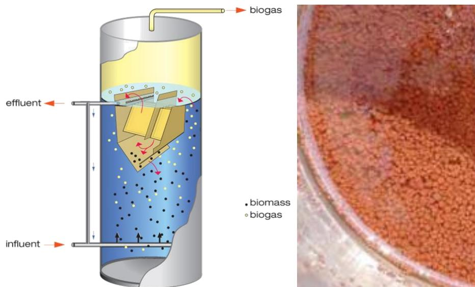
Figure 6: Schematic set-up of the ANAMMOX<sup>®</sup> process (left)<sup>4</sup> and the biomass content of this reactor set-up (right)<sup>5</sup>.
