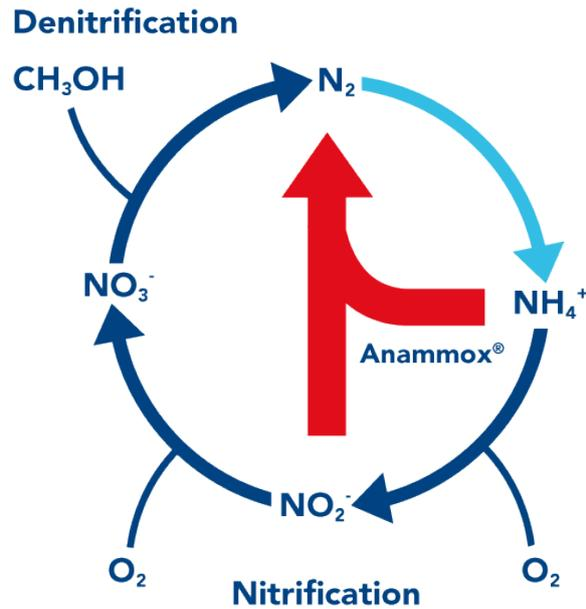
Figure 3: Nitrogen cycle with anammox pathway<sup>1</sup>
