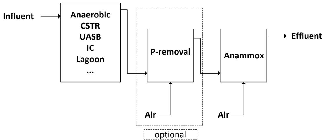
Figure 11: Principal side-stream setup and anammox positioning.
