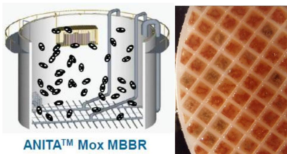
Figure 7: Schematic set-up of the ANITA<sup>™</sup> Mox process (left)<sup>6</sup> and the biomass content (right)(left)
