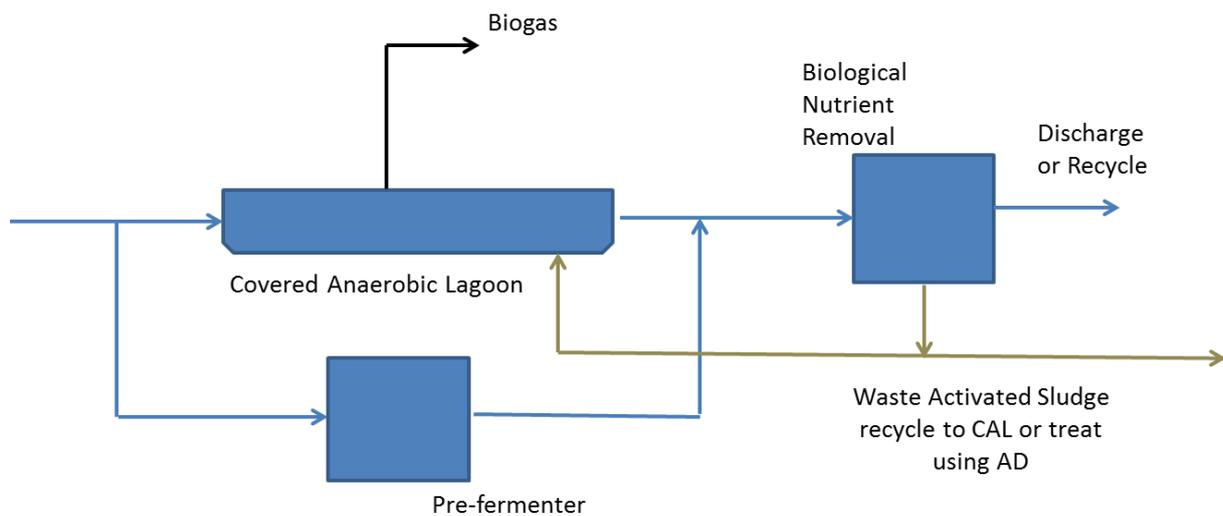
**Figure 19: Process flowsheet representing a covered anaerobic lagoon followed by nitrification/denitrification in an SBR. The process is similar to that presented in ENV.044.**
