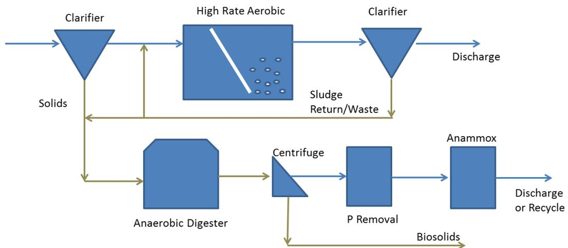
Figure 18: High rate aerobic wastewater treatment and anaerobic digestion with anammox integrated for treatment of side stream AD centrate (A.ENV.0150)
