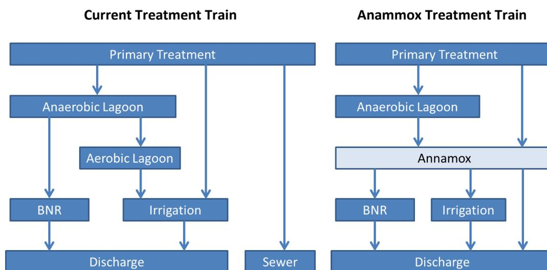
Figure 16: Integration of anammox into current process treatment train after primary treatment or anaerobic treatment
