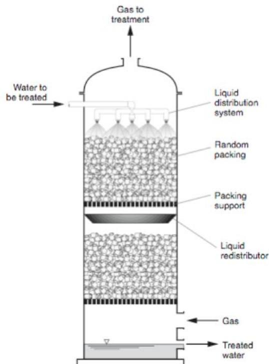
Figure 15: Schematic stripping tower where air is pumped into the bottom of the tower to remove volatile components of contaminated water added to the top of the tower (Crittenden et al 2005).
