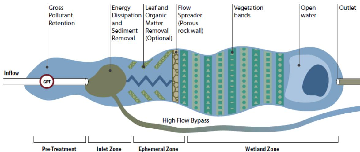
Figure 14: Schematic set-up of a typical constructed wetland (from *Constructed wetlands systems design guidelines for developers 2005*).
