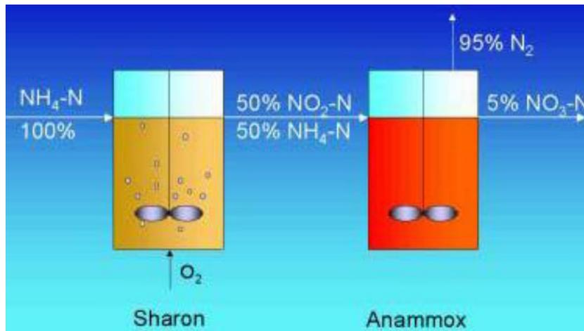
Figure 5: Schematic set-up of a two-step system, including a SHARON<sup>®</sup> and ANAMMOX<sup>®</sup> reactor<sup>3</sup>
