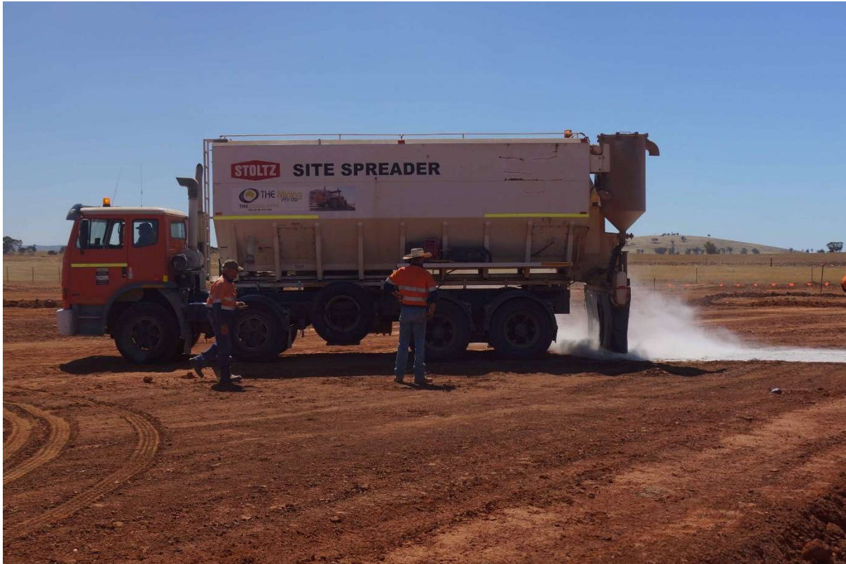
Figure 1. Spreader applying lime to the pens surface. Source Premise Agriculture
