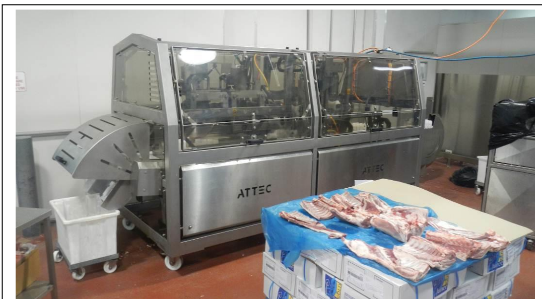
Figure 9. Lamb Whole Barrel Machine in trial position. Smallest and the largest whole barrels cut straight after power up are shown.
