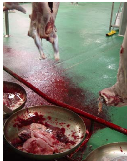
Carcase travelling away from the pan system at 45 degrees. If red offal operator becomes held up there is still time for him to remove the offal without too much manoeuvring.
