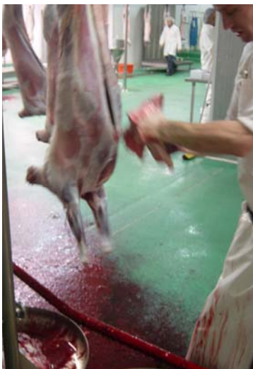
Carcase travelling away from the pan system at 45 degrees. If red offal operator becomes held up there is still time for him to remove the offal without too much manoeuvring.
