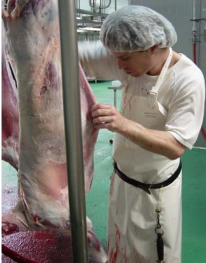
Operator removing red offal carcasses positioned central to white offal pan with red offal trailing.
