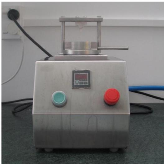
**Figure 1. The G1 tenderometer**
