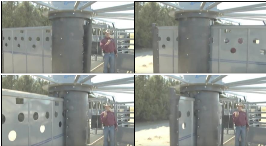
Figure 6.5 Automated turret. (Source: Youtube 2017; http://www.catagra.com ) illustrating the rotating and shuttling motion of the gate.
