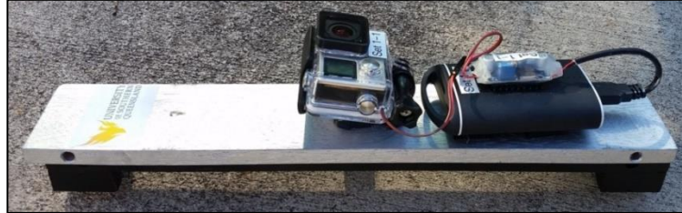
Figure 1. Detail view of a single wireless camera unit.
