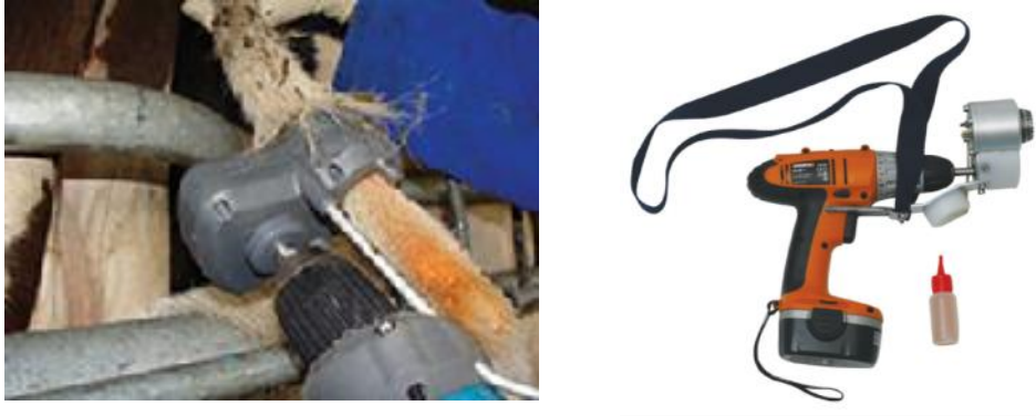
Figure 6.13 TailWell2™ - Power Tail Trimmer drill attachment for trimming tails (Shoof International Ltd. New Zealand).
