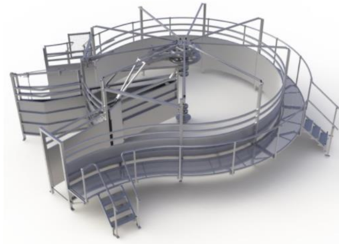
Figure 6.3 Curved tub configuration of a Crowd Pen. (Davis and Janke 2016)
