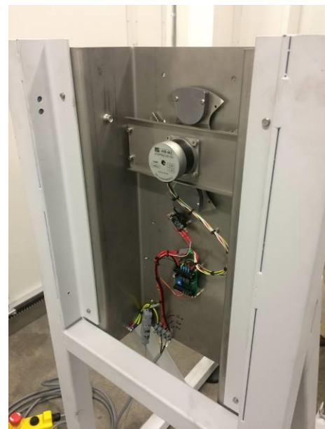
Figure 1: X-ray source, or tube, mounted in position (Left). Opposite side of tube mount, showing stepper controlled lead shutter and filter wheel (Right)
