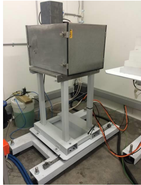
Figure 3: Hamamatsu high speed camera mounted to detector box, with lead shroud removed (Left). Full view of detector box and stand, showing horizontal positioning axis, phosphor panel fitted to front, and leaded camera shroud in place at top (Right).
