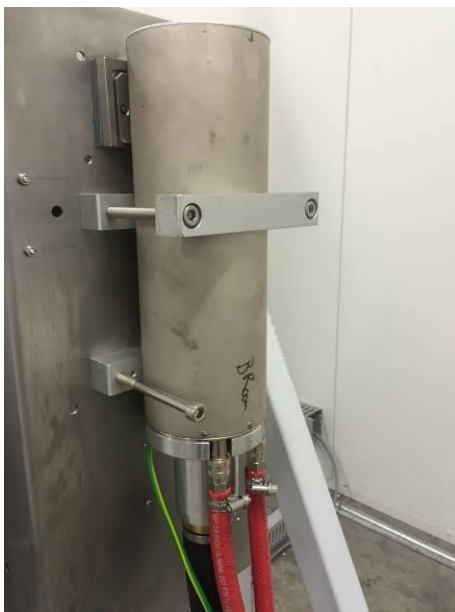
Figure 1: X-ray source, or tube, mounted in position (Left). Opposite side of tube mount, showing stepper controlled lead shutter and filter wheel (Right)
