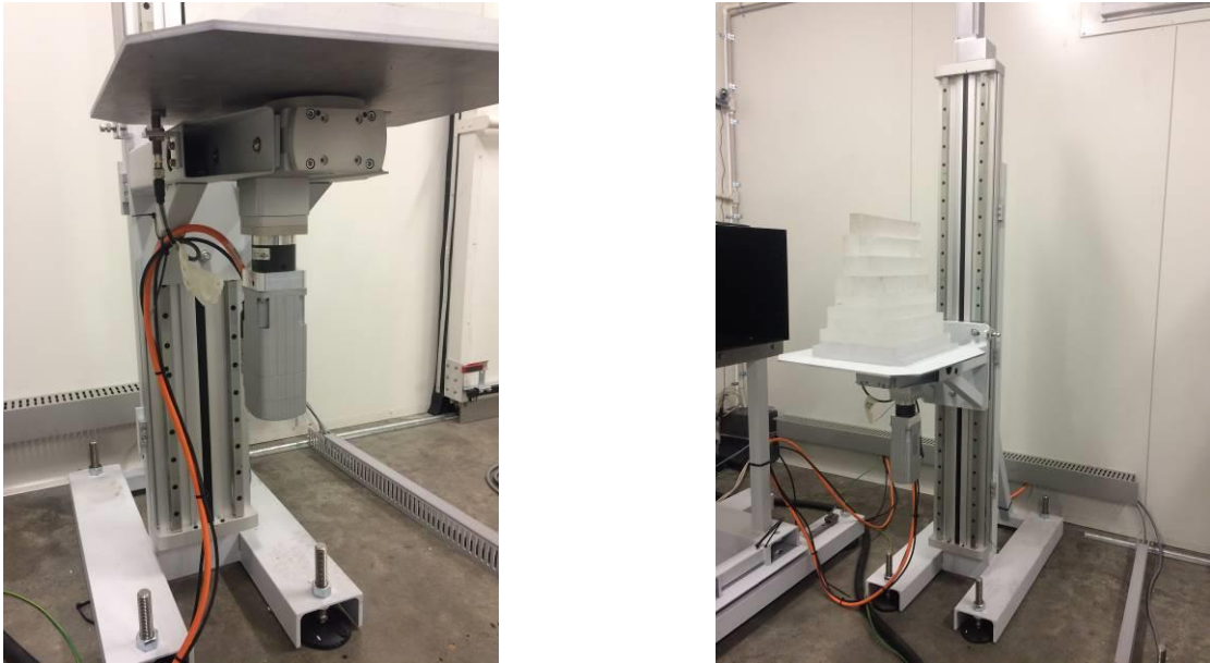
Figure 2: Underside of table showing rotational servo drive and reduction gearbox (Left). Full view of table, with servo motor at top for driving vertical axis (Right).
