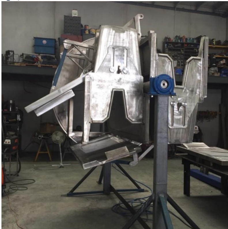
Figure 5: View of the neck capture, side and 'top' doors opened to allow ejection of the animals when inverted. Image taken during workshop construction. In this image, the upright side is to the right, and the inverted side to the left.
