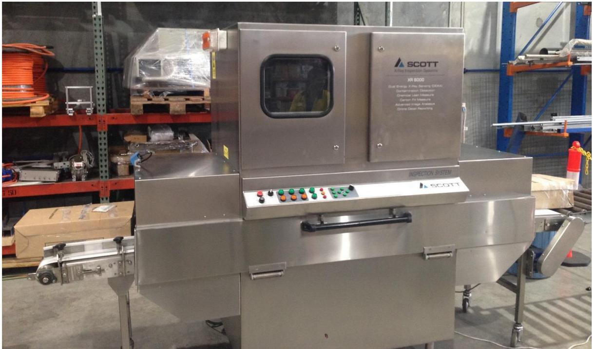
Figure 3: XR8000 inspection prototype platform with an upgraded detector inside.
