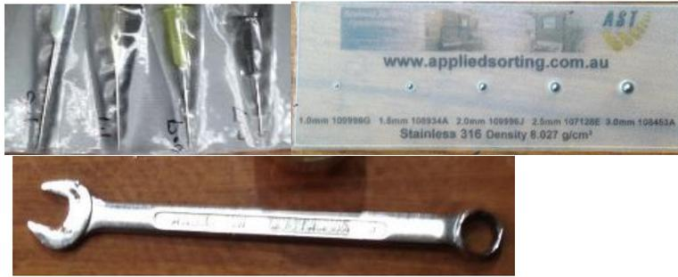
Figure 26: Stainless steel and metals used for contaminant inspection.
