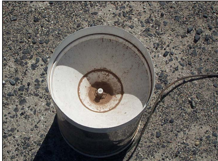
Figure 2. A Dust Blockage of a Rain Gauge.
