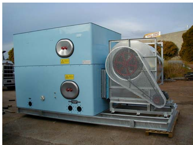
Figure 6. Forced draft cooling tower.
