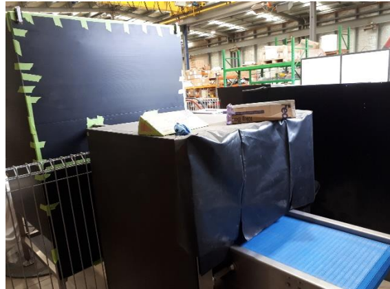
Fig. 3 Infeed conveyor and Sick ruler scanner housing
