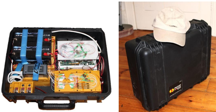
Figure 3. Battery-operated prototype scanner. (left) Internal components. (right) Assembled system in a waterproof carrycase (cap is shown to give an understanding of size).
