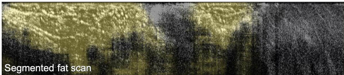
Figure 6. (top) IMF needle scan (scans are approximately 8mm x 1mm, length x depth). (bottom) Results of automated analysis. Fat is coloured yellow.
