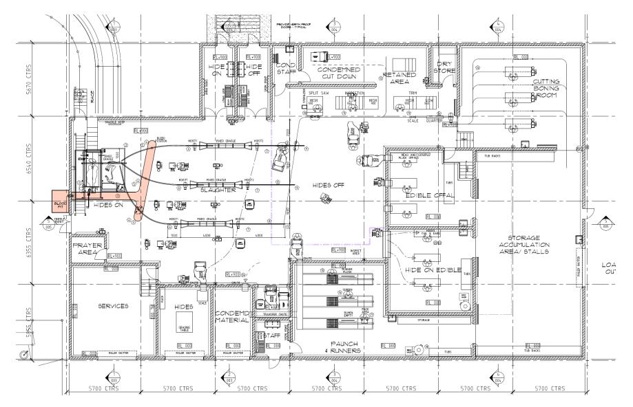
Figure No. 4: Process Layout for combined bed and rail dressing process
