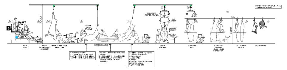
Figure No. 6: System B: Combines bed and rail dressing system
