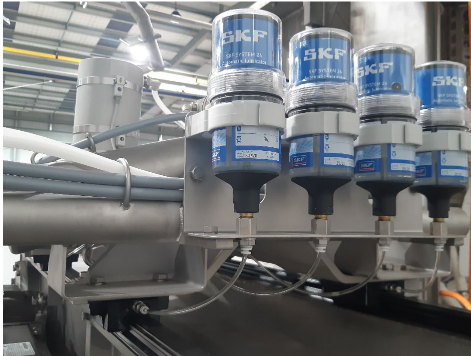
Figure 26: Adaption module for electro-mechanical lubrication mounting for key assemblies. Single axis arrangement.
