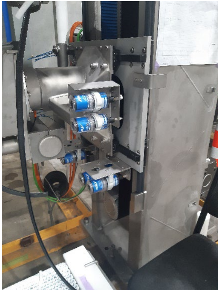
Figure 24: LEAP III Saddle station Additional examples of adaption concepts throughout the cutting heads.
