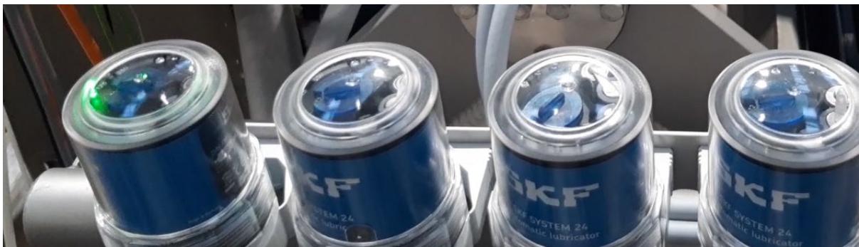
Figure 20: New Single Point Lubricators have LED status lights that flash every 5 minutes clearly indicating to the operator or maintenance staff which lubrication points require attention.
