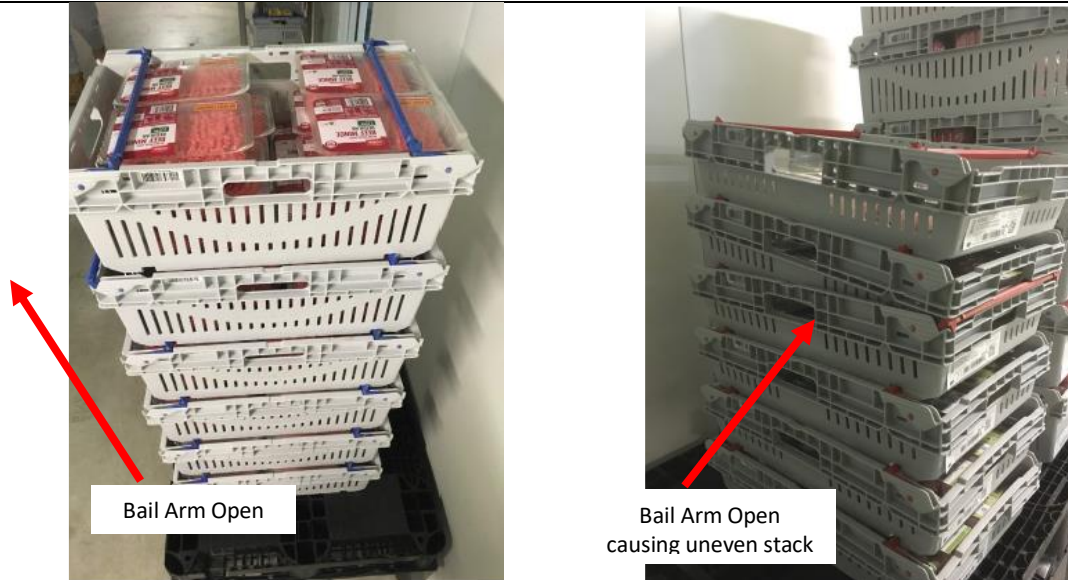
Photo 4: Improperly stacked trays or lifted bail arms cause faults in the system.
