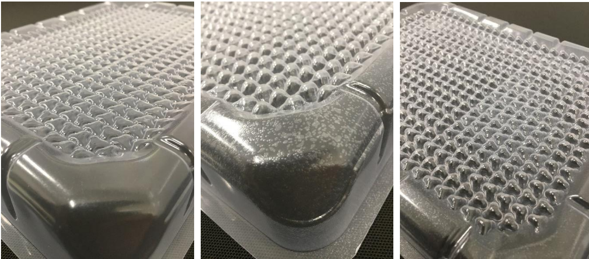
Photo 15: Trays formed during the trial – Inconsistent forming quality
