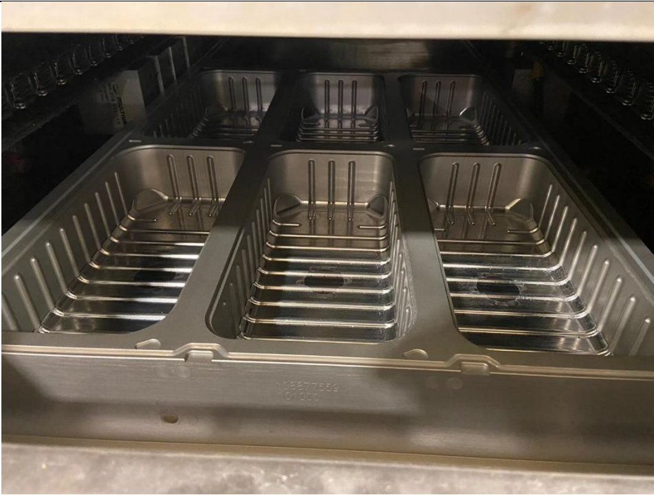
Photo 1: New Die Inserts to add extra Ribs
