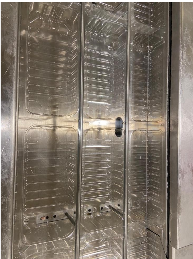
Photo 2: New and Improved Trays with additional ribs for rigidity improvement
