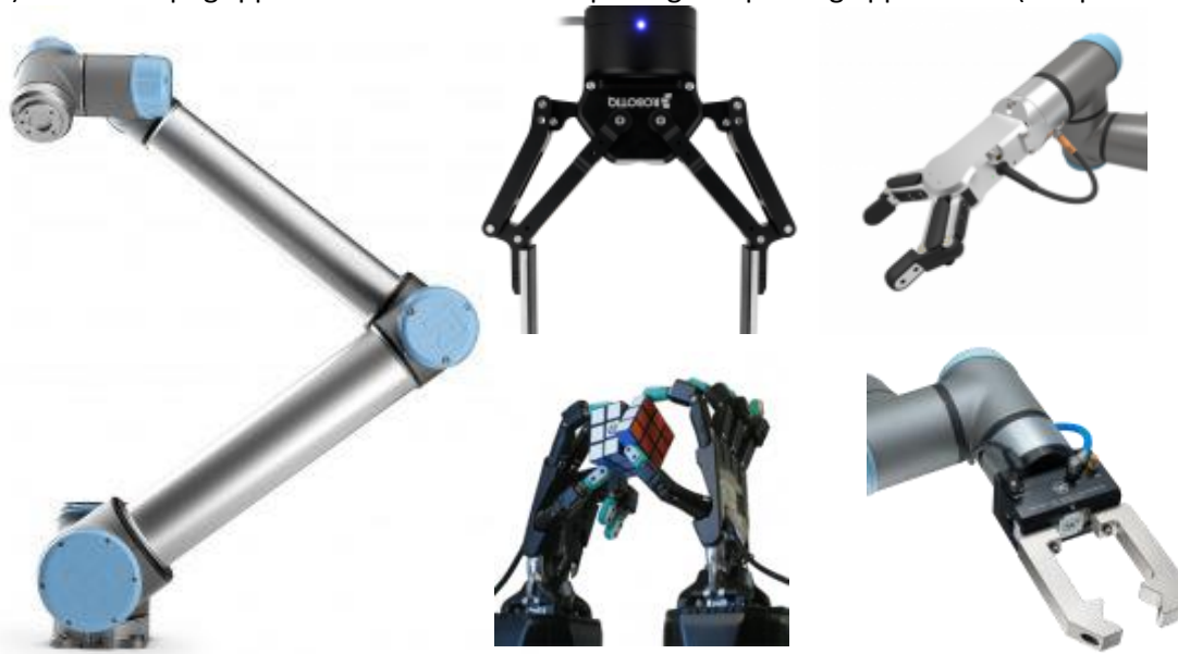
Photo 1: Collaborative robot & grippers proposed for picking and placing raw red meat cuts and packaged product.
