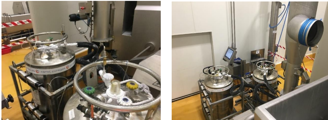
Photo 16: Portable nitrogen vessels used for production trials
