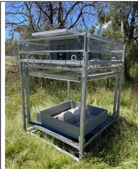
**Figure 11.5a. Suspension block weigher**
