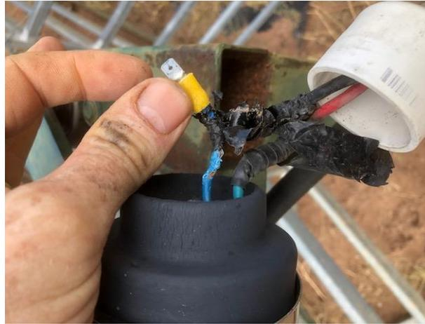
**Figure 11.7. Bird damage to exposed wires on walk-over weighing unit**
