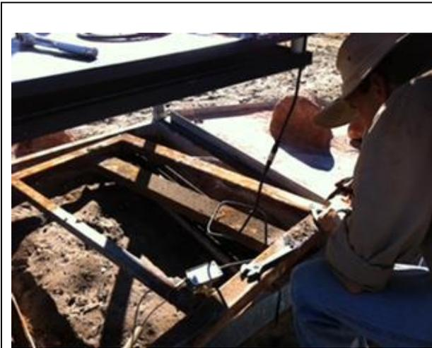
**Figure 11.3. Severe rust on the load bars beneath the weigh platform of a lick-block weigher**
