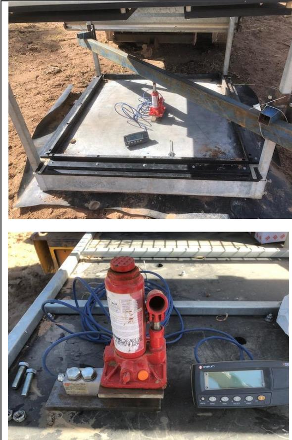
**Figure 11.6. Use of hydraulic jack and calibrated load cell to calibrate lick-block weigh platform.**
