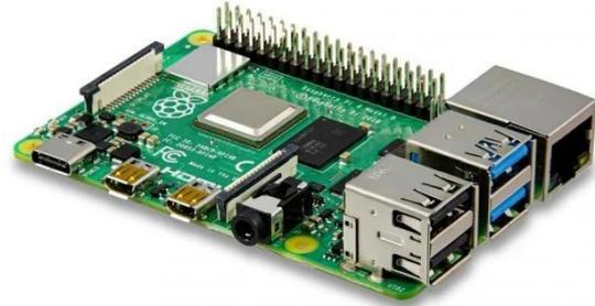
**Fig 11.11 Raspberry pi Single Board Computer. These operate in WoW and Block weigher units and can process/transform data prior to sending, can be modified remotely and set up a local WiFi network**
