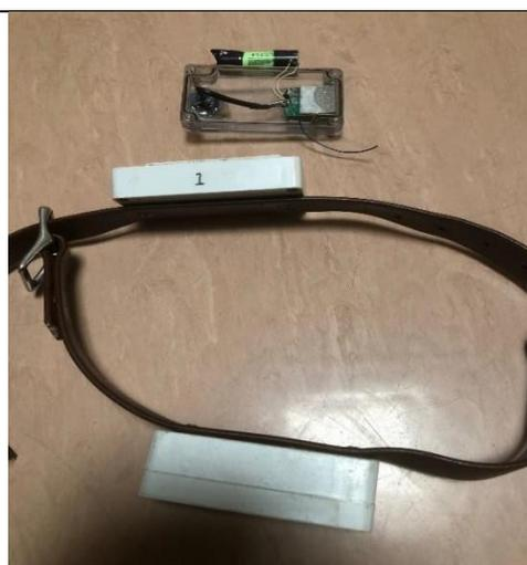
Figure7. 2. GPS collar as used at Burleigh 2<sup>nd</sup> box is for counterweight to keep GPS tracker high on the neck and can also house auxiliary batteries.
