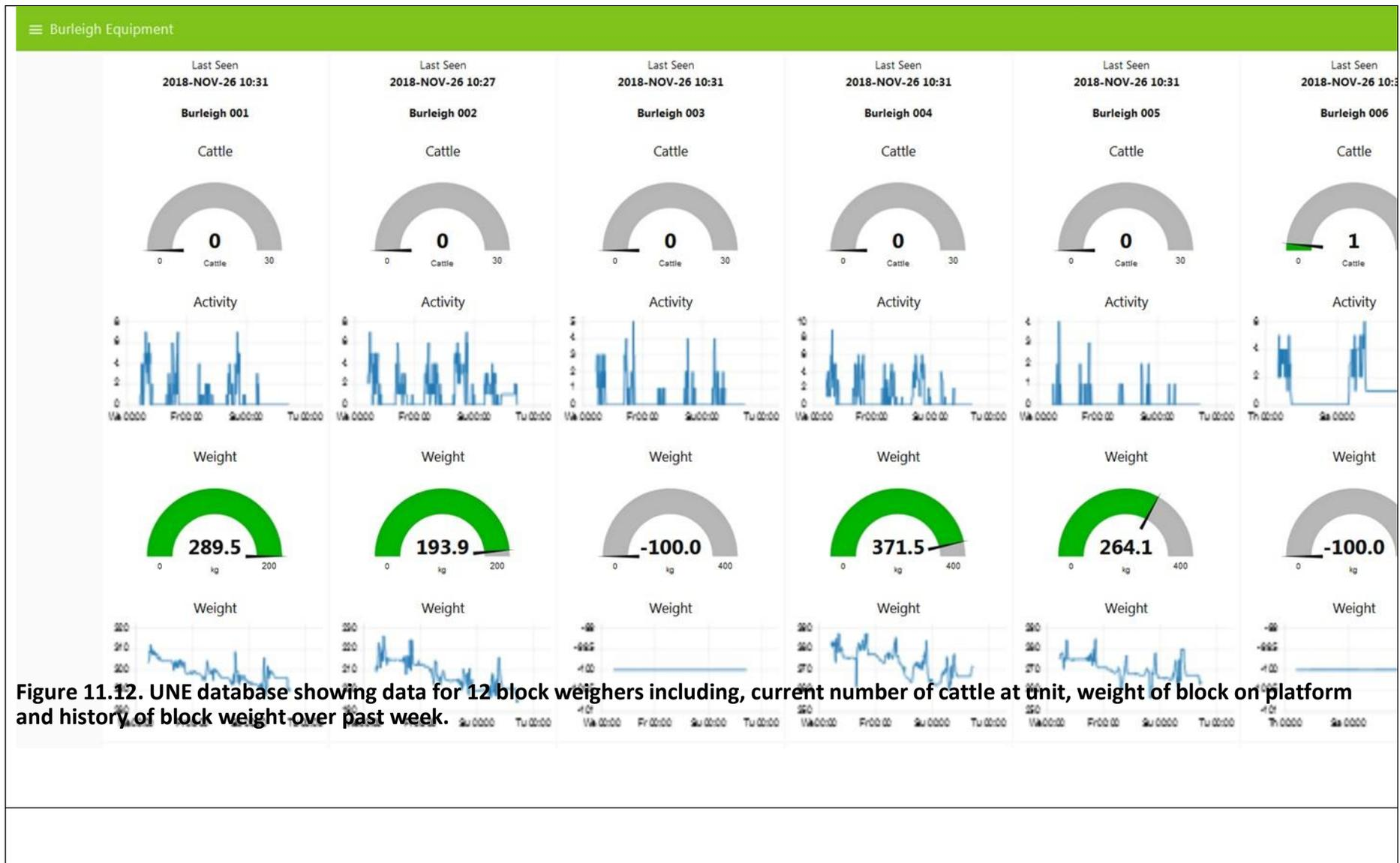
Figure 11.12. UNE database showing data for 12 block weighers including, current number of cattle at unit, weight of block on platform and history of block weight over past week.
