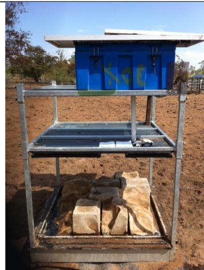
**Figure 11.4. Hot-dipped galvanised block-block weigher replacement unit**
