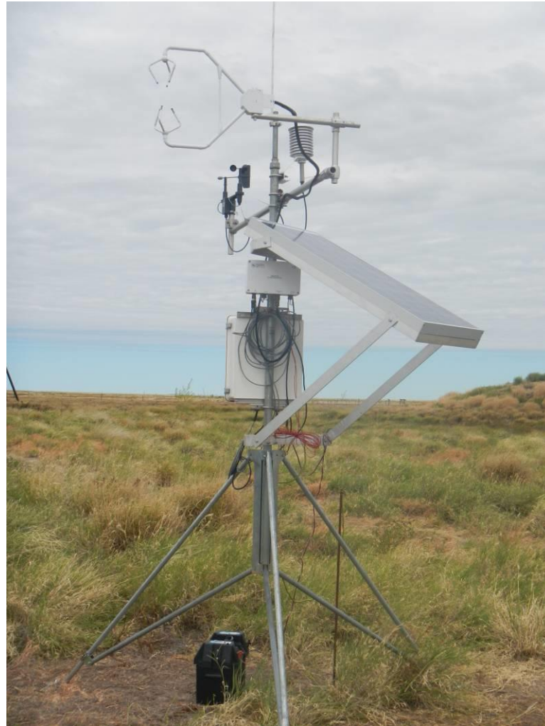
Fig. 3 A micrometeorological mast equipped with a three-dimensional sonic anemometer, cup anemometer, wind vane and temperature/humidity sensors was located upwind and adjacent to the source area defined for the AACo Brunette Downs campaign.
