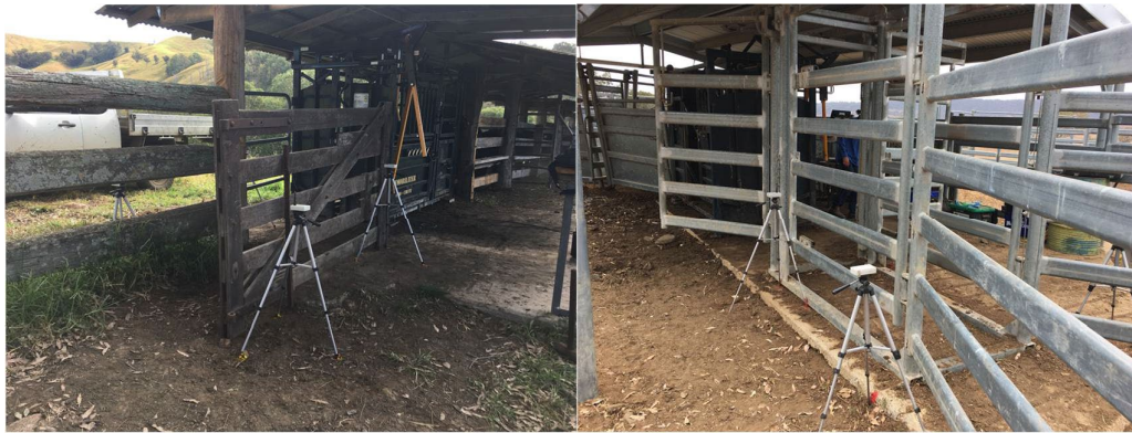
Figure 4. Flight speed testing setup as used at Co-operator Herd 3 (left) and Herd 1 (right) cattle handling facilities.
