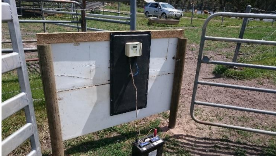
Figure 6 - The timber section of fence with Sapien Technology PedigreeScan panel reader in place at site 1
