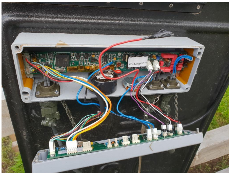
Figure 38 - Disconnecting the beeper on Allflex panel reader
