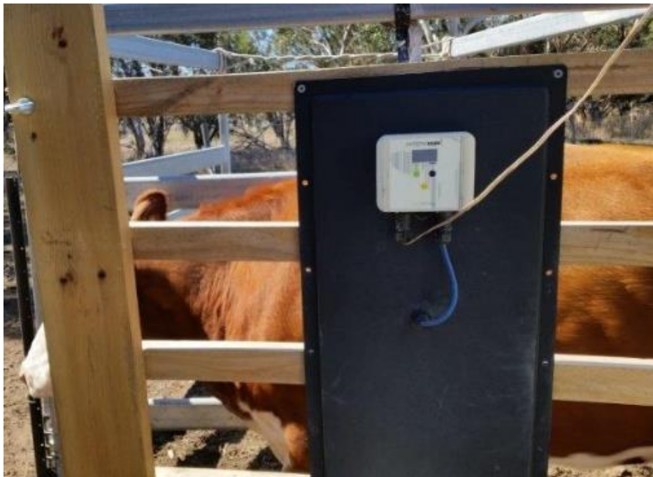
Figure 22 - Site 2 2015 - cow travelling pass the Sapien Technology PedigreeScan panel reader demonstrating the height of recording for cows
