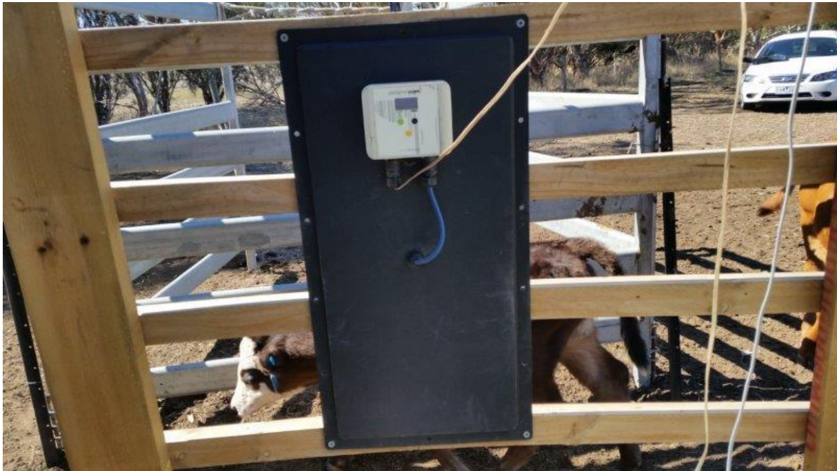
Figure 21 - Site2 2015 - calf travelling past the Sapien Technology PedigreeScan panel reader demonstrating the height of recording for calves
